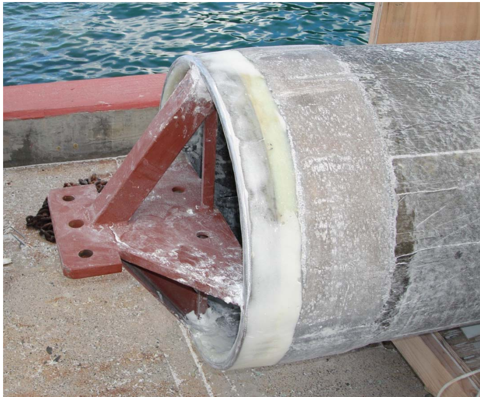
Figure 262. Termination Added to Lower End of CWP
