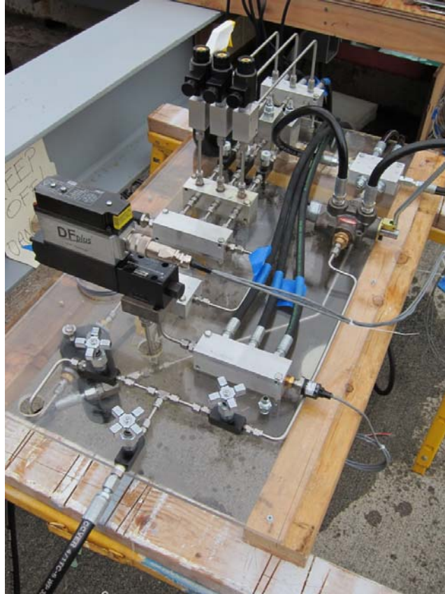
Figure 269. Hydraulic Valves and Controllers
