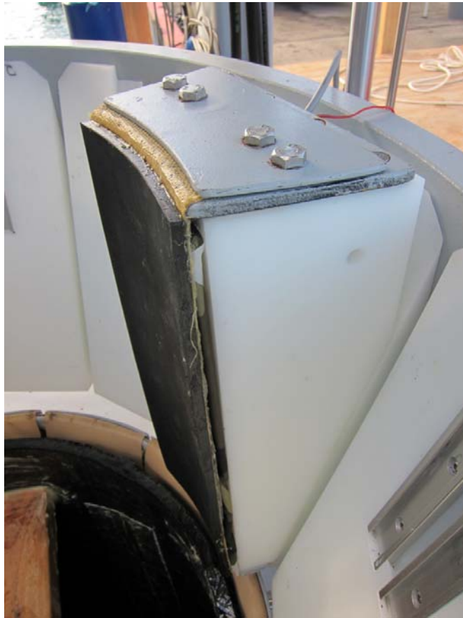
Figure 252. Wedge with Gel Pad, Tension and Friction Layers.
