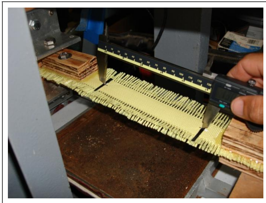
Figure 201. Testing Elasticity of Kevlar Fabric
