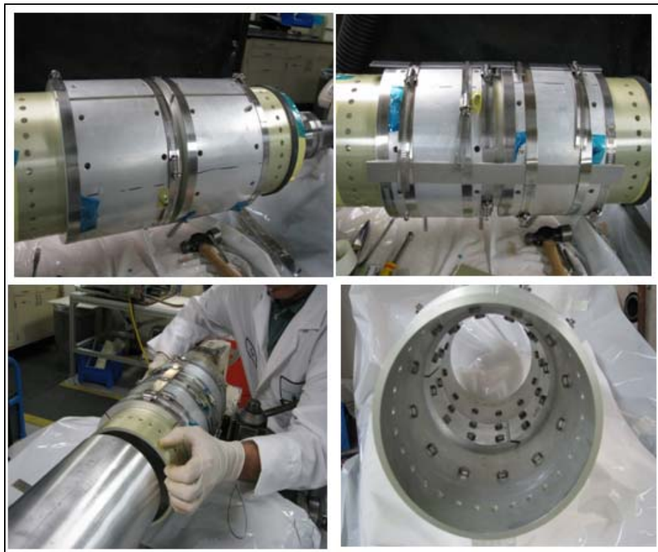
Figure 83. Add Outer Backing Plates, Remove from Layup Mandrel
