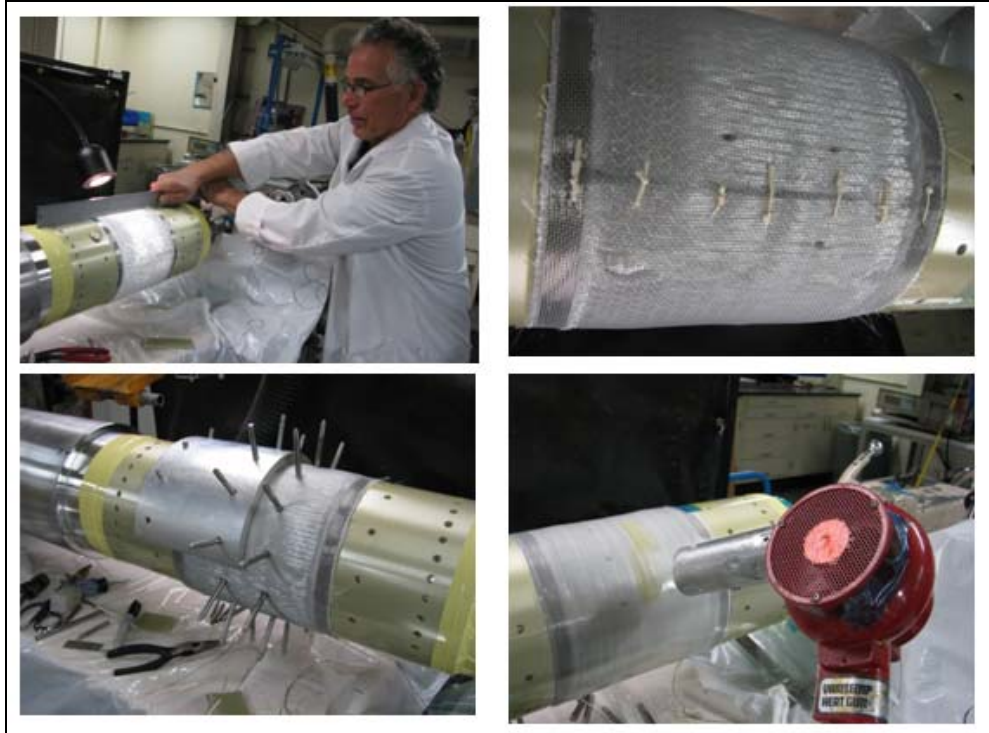
Figure 82. Add Resin Distribution Medium (RDM)
