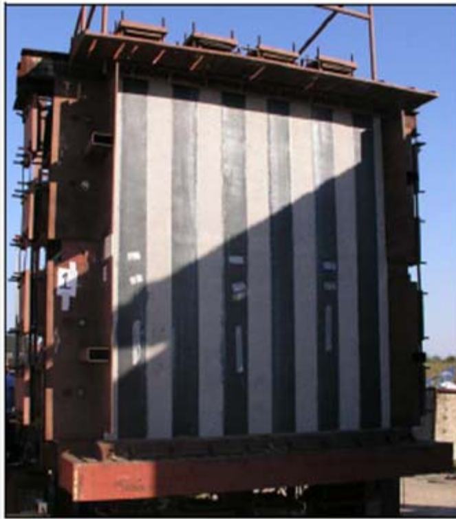
Test walls in BakerRisk shock tube
