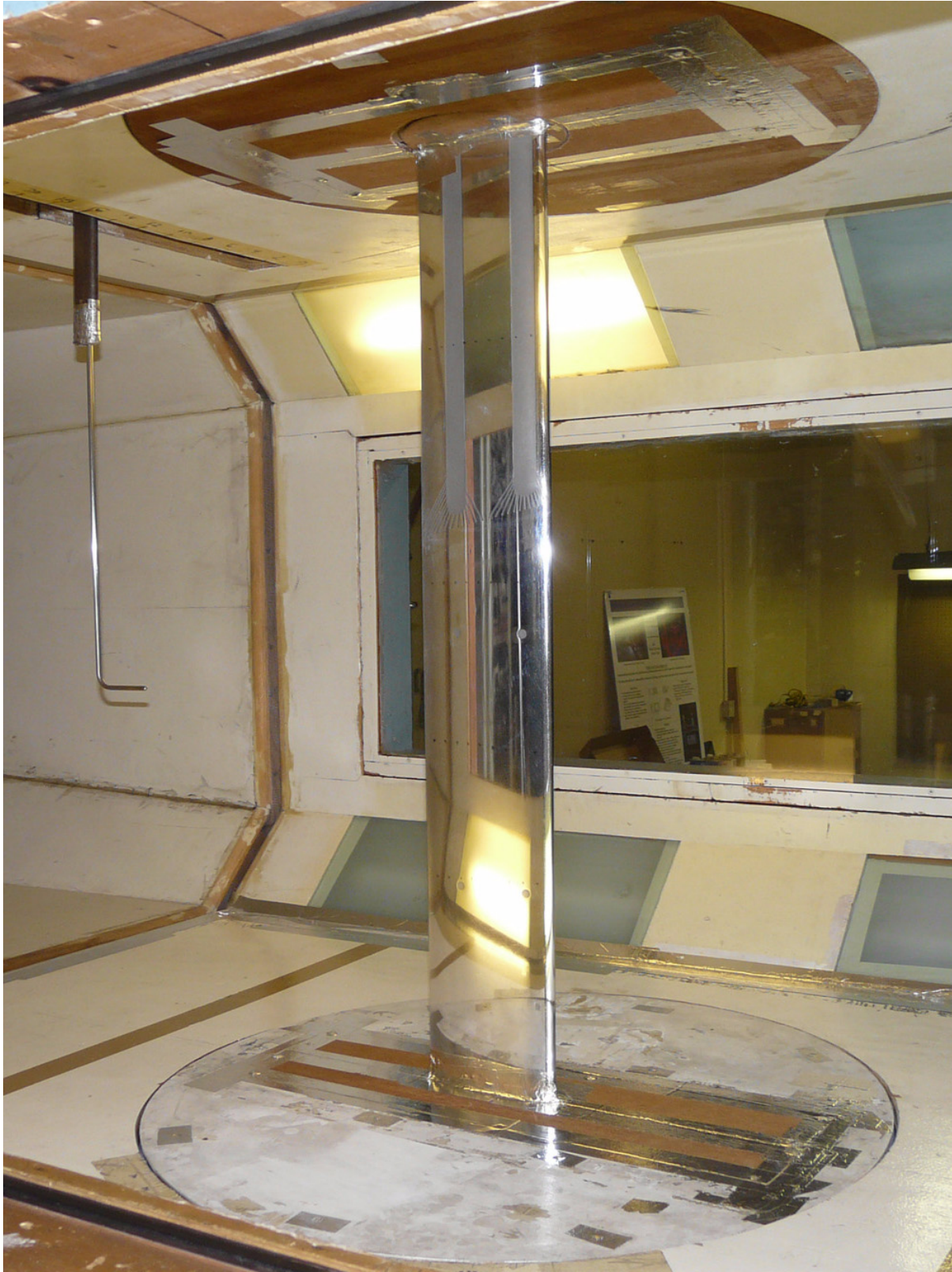
Figure 2.- S407 airfoil model and wake-survey probe mounted in test section.
