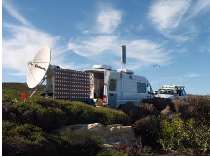
Figure 15: Setup of sea clutter collection. Receiving channel 16 is closest to the transmitter on the top of the van. Note that the dish antenna belongs to another radar and is irrelevant to this report.
