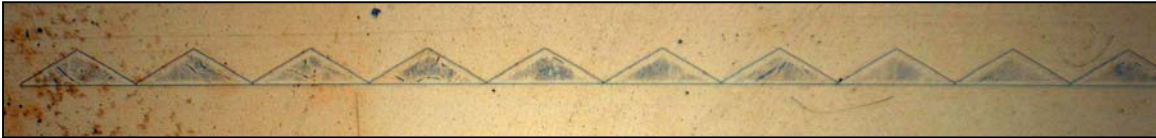
Figure 5.1 – The poled prisms of First Generation Chip 1 exhibit excellent quality.
