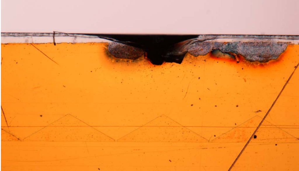
Figure 5.7 – Damage from dielectric breakdown of the air between the top electrode of FCG-1 and the aluminum mount.
