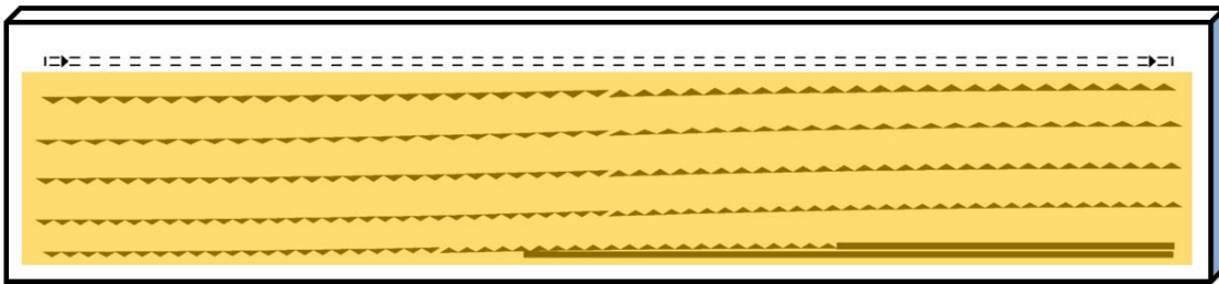
Figure 3.24 – The finished EOBS chip with gold electrodes.
