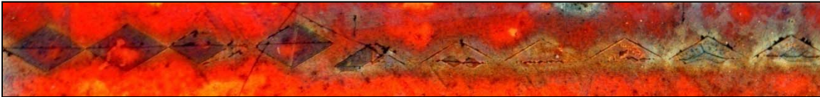
Figure 5.2 – The poled prisms of First Generation Chip 2 exhibit poor quality. [The discoloration is due to tarnishing of the gold electrode.]
