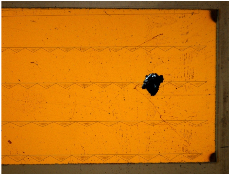
Figure 5.30 – Damage from bulk dielectric breakdown of SGC-1.
