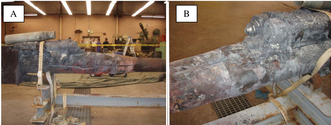
Figure 1 Failed 100-mm gun tube after incident, 65” and 60” long cracks in images A and B respectively
