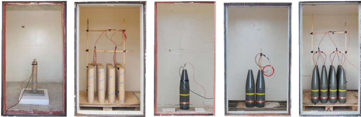
Figure 2. The charge configurations used in Kasun-III were 6.9 kg uncased, 100 kg uncased, one 155 mm shell, four 155 mm shells and sixteen 155 mm shells (from left to right).
