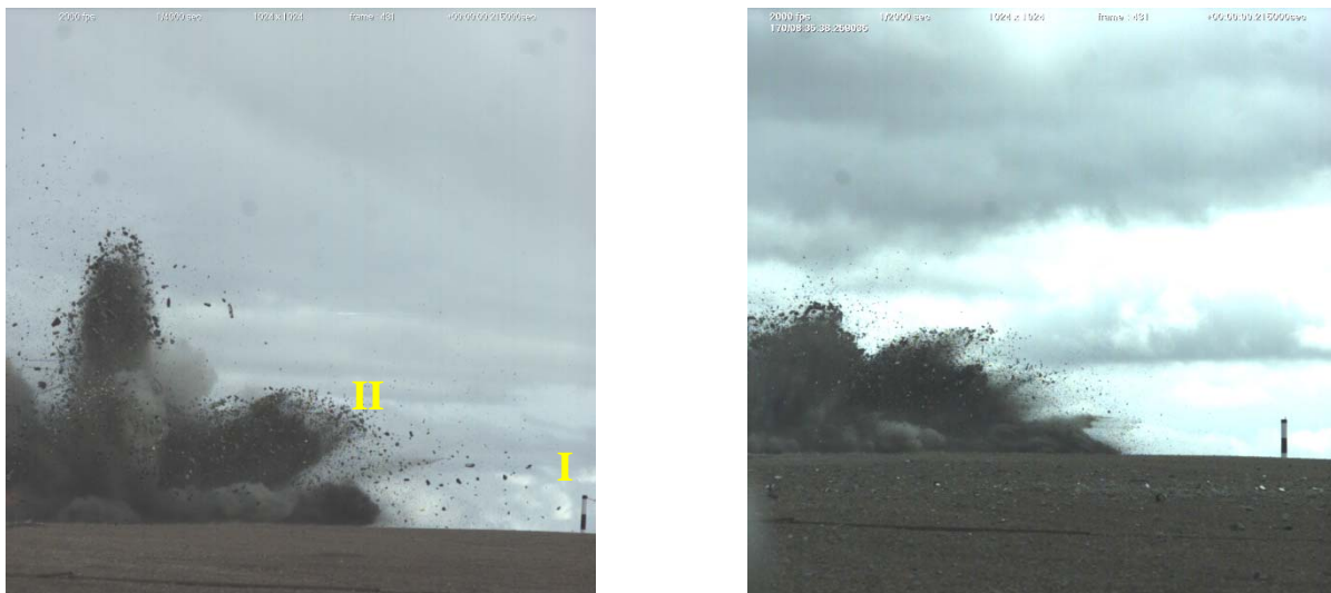
Figure 5. Still images from the high speed video footage showing the debris throw from 6.9 kg uncased charge (left) and 1x155 mm shell (right). The images are at identical elapsed time since detonation.
