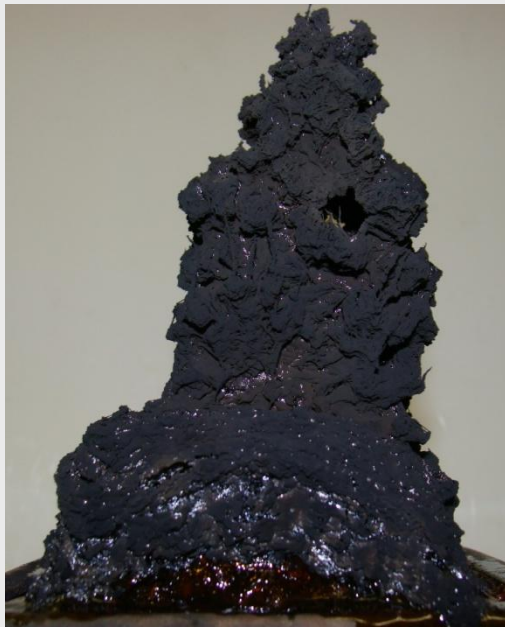
5 mm PC sample after 160 s at 75 \text{ kW m}^{-2} .
