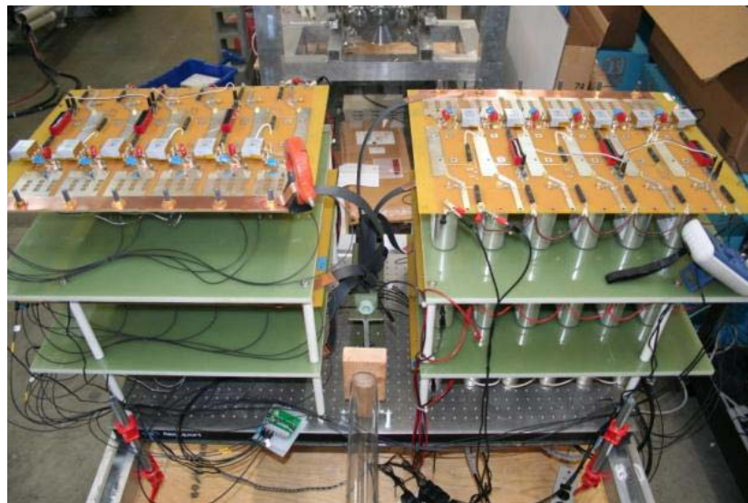
Figure 2. Six staged MLP system (Shown are solid-state switching, parallel capacitors, fiber-optic trigger and data acquisition unit, and macron launcher) 3
