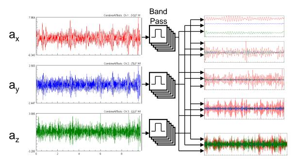
Rainflow cycle count the filtered acceleration data to yield 3 damage vs frequency plots for x,y,z:
