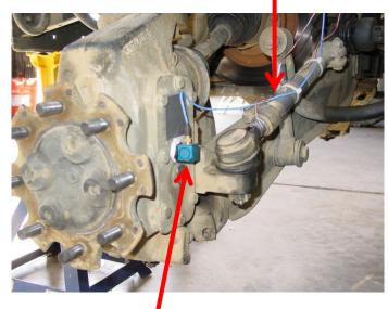
Triaxial accelerometer located at left front wheel
