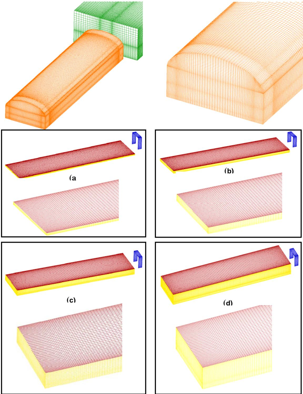
FIGURE 6. 3D Computational Surface Grid with Four Weights: (a)  $1.0\text{E}5$  lb ( $4.53\text{E}4$  kg), (b)  $2.5\text{E}5$  lb ( $1.13\text{E}5$  kg), (c)  $5.0\text{E}5$  lb ( $2.27\text{E}5$  kg), (d)  $1.024\text{E}6$  lb ( $4.65\text{E}5$  kg).
