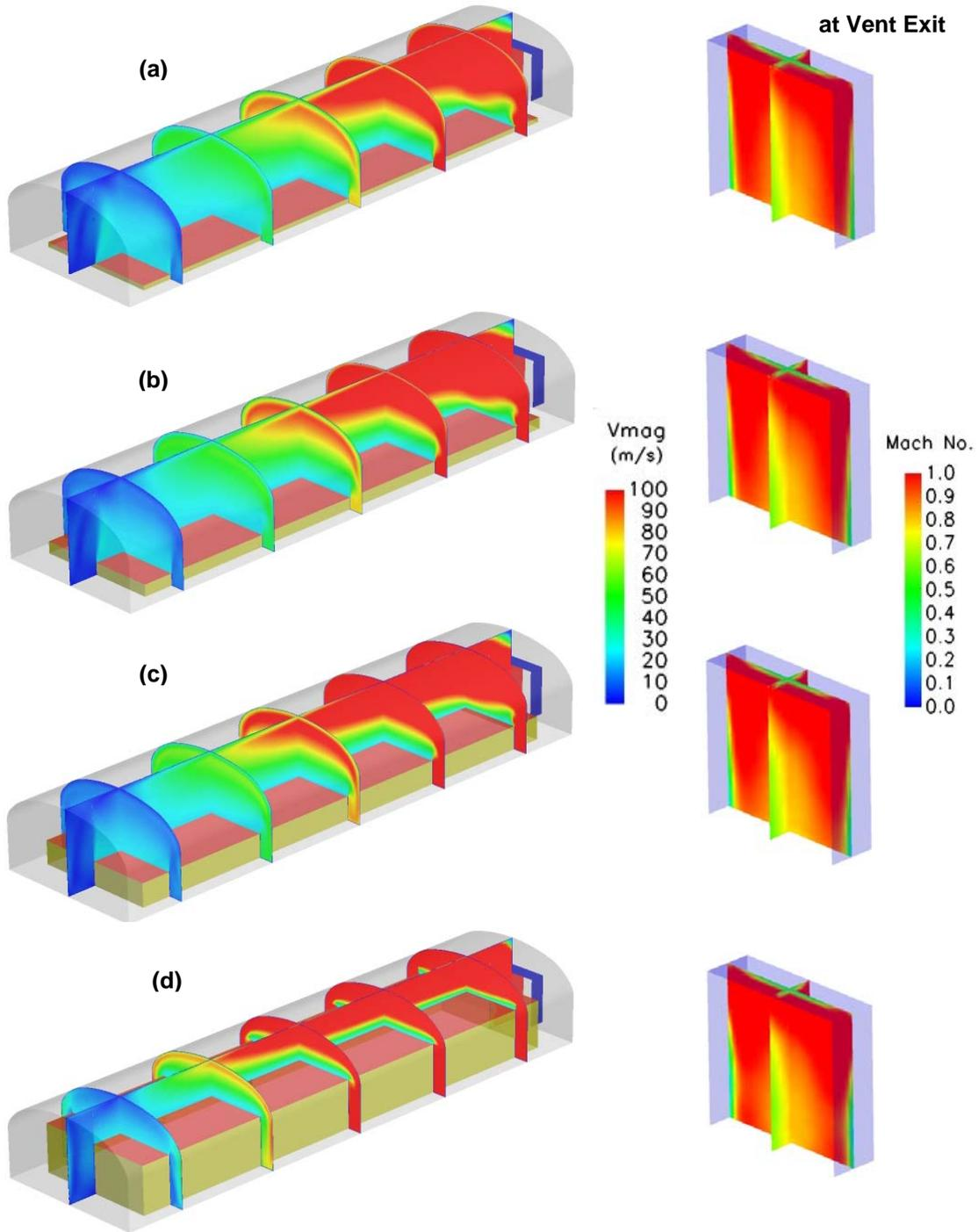
FIGURE 11. Velocity Magnitude and Mach Number Contours With 200 Percent Nominal Burning Surface Area for Four Weights: (a)  $1.0E5$  lb ( $4.53E4$  kg), (b)  $2.5E5$  lb ( $1.13E5$  kg), (c)  $5.0E5$  lb ( $2.27E5$  kg), (d)  $1.024E6$  lb ( $4.65E5$  kg).
