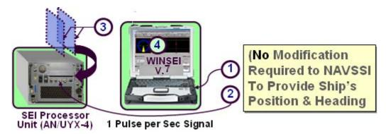
The two components within the AN/SSX-1 system that require minor modification to enable Sea Node capabilities are the AN/UYX-4 SEI Processor unit (left in the Figure above) and the laptop computer, which requires that the WinSEI software be upgraded from version 5.2D to version 7.2. The following steps are required to implement the changes:
