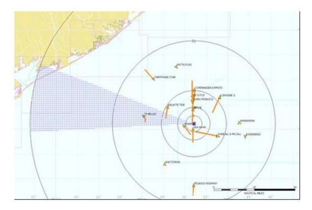
The cross-hatched triangle represents the ES system's antenna pointing angle and beamwidth. The orange tracks close to the own-ship position are time-sequenced AIS contacts. The displayed AIS contacts can be managed by the operator to enable shorter or longer persistence of the tracks. Detailed geographic information is depicted dynamically as the ship is underway. ES antenna tracking can be set to automatic. The viewing radius is operator-controlled.
