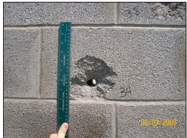
Figure 6 – Front (left) and Back (right) of CMU Wall After Impact (No Perforation) by 1.125" (28.58mm) Steel Impactor on Unreinforced Cell
