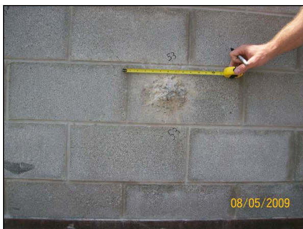
Figure 7 – Front (left) and Back (right) of CMU Wall After Impact (No Perforation) by 5" (127.00mm) Concrete Impactor on Reinforced Cell
