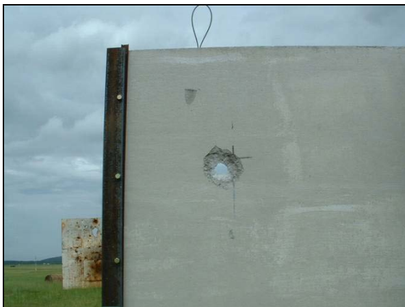
Figure 4 – Front (left) and Back (right) of Reinforced Concrete Wall After 2.5" (63.50mm) Steel Impactor Perforation
