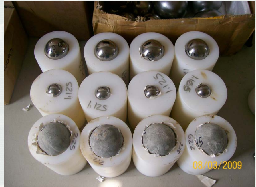
Concrete (bottom row) and Steel (top & middle row) Impactors in Sabots
