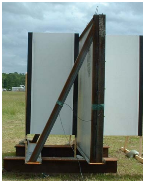
Figure 3 – Reinforced Concrete Wall Test Setup
