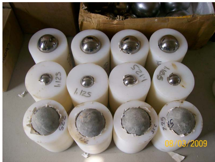
The sizes of the impactors were determined based on SAFER KE bins 3 through 7 (TP 14, 2009) and the average fragment mass corresponding to the average SAFER KE for each bin (see Table 5). Impactor weights were adjusted slightly depending on commercially available steel spheres and concrete spherical molds (see Table 6).
