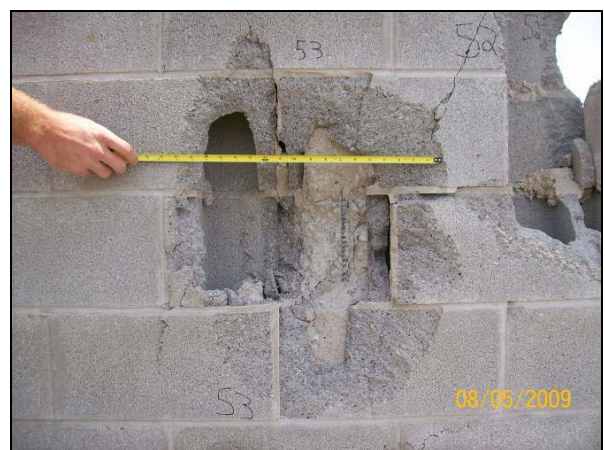
Figure 7 – Front (left) and Back (right) of CMU Wall After Impact (No Perforation) by 5" (127.00mm) Concrete Impactor on Reinforced Cell
