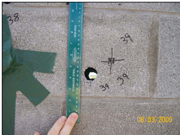
Figure 6 – Front (left) and Back (right) of CMU Wall After Impact (No Perforation) by 1.125" (28.58mm) Steel Impactor on Unreinforced Cell
