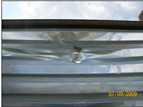
Figure 5 – Front (left) and Back (right) of Corrugated Steel Panel After Impact (No Perforation) by 3" (76.20mm) Concrete Impactor
