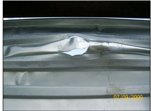
Figure 5 – Front (left) and Back (right) of Corrugated Steel Panel After Impact (No Perforation) by 3" (76.20mm) Concrete Impactor
