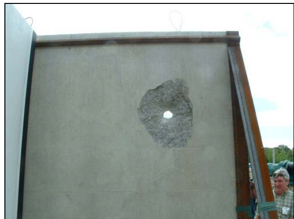
Figure 4 – Front (left) and Back (right) of Reinforced Concrete Wall After 2.5" (63.50mm) Steel Impactor Perforation
