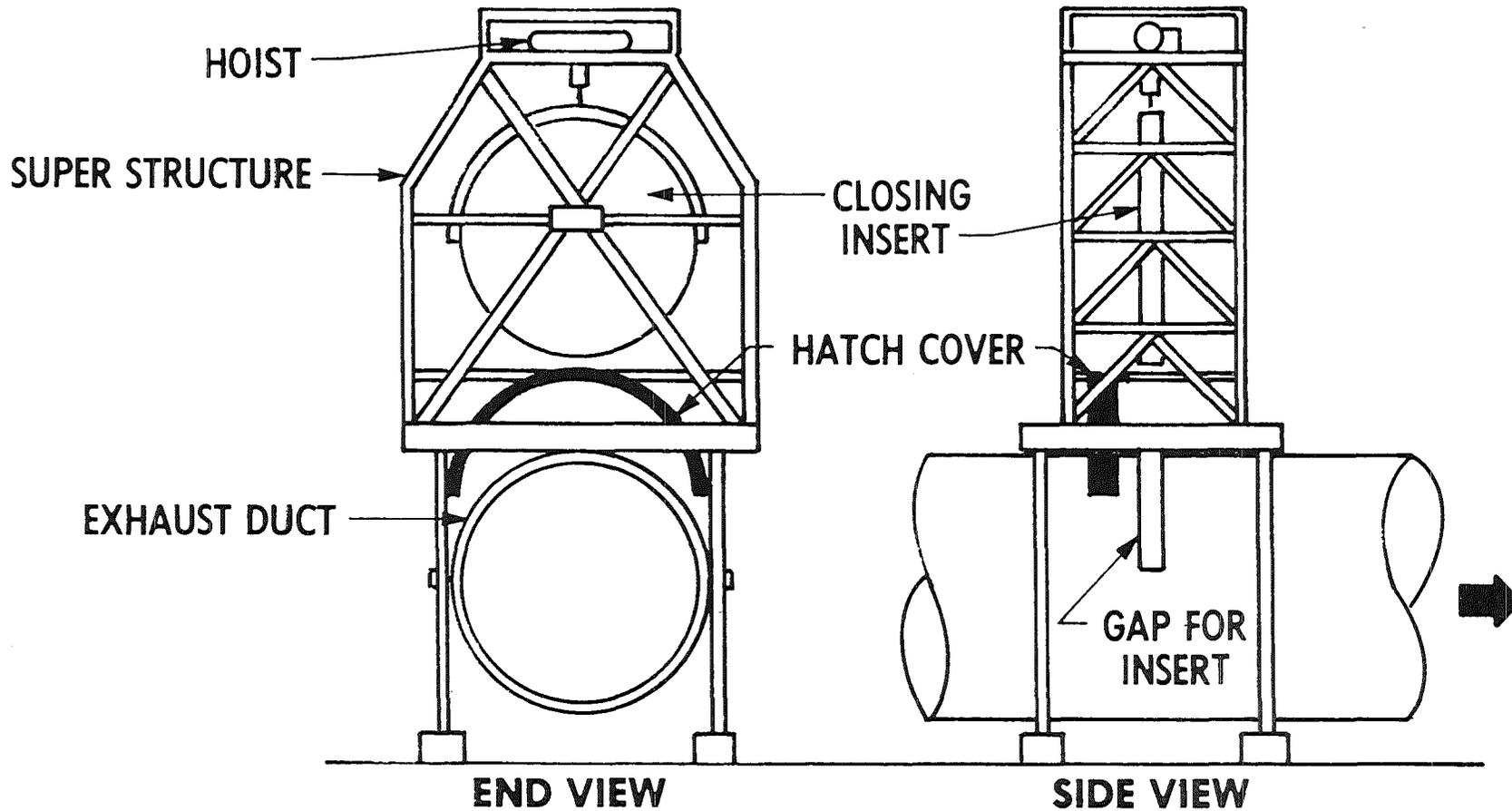
**NOTE: VALVE IS SHOWN WITH CLOSING INSERT AND HATCH COVER IN STORED, INOPERATIVE POSITION**
