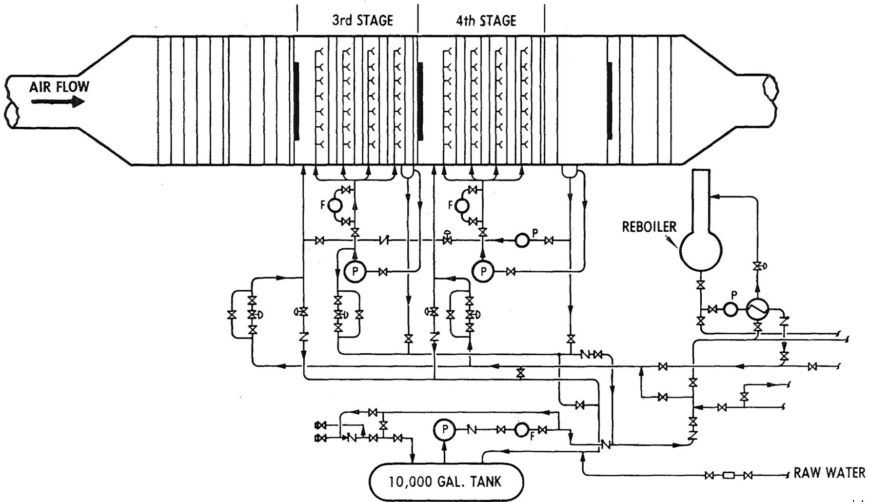
Figure 11. Cooler RCl De-icing Spray System.
