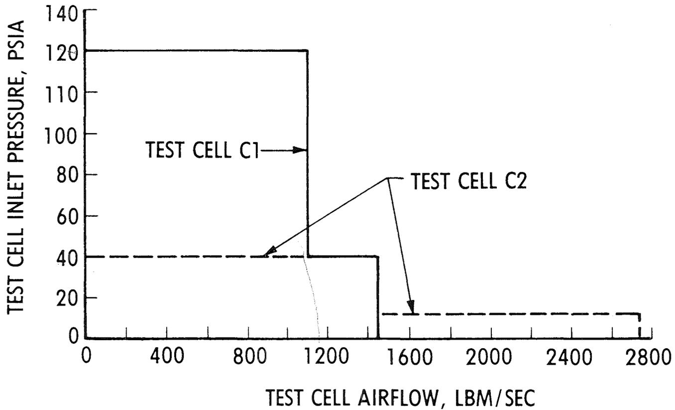
Figure 5. Air Supply System Pressure Capability.
