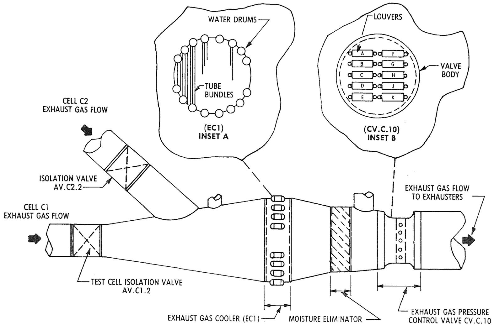
Figure 17. Exhaust Gas System Transition Section Illustration.
