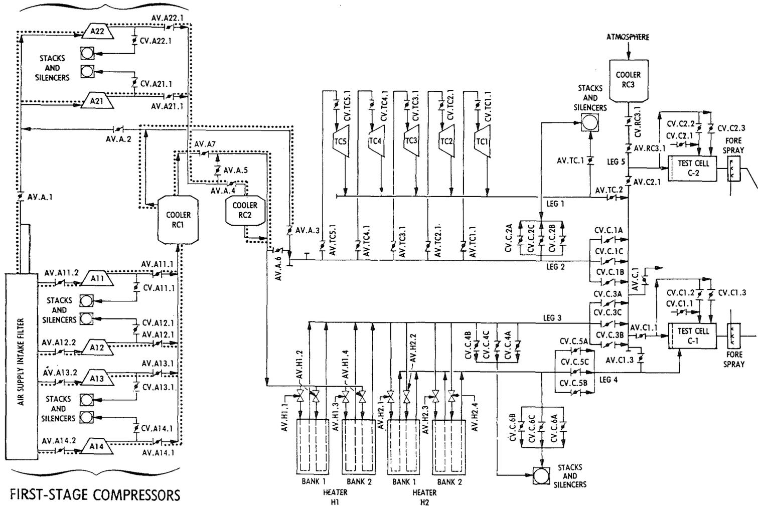
Figure 27. Air Supply Compressor Single-Stage Configuration.
