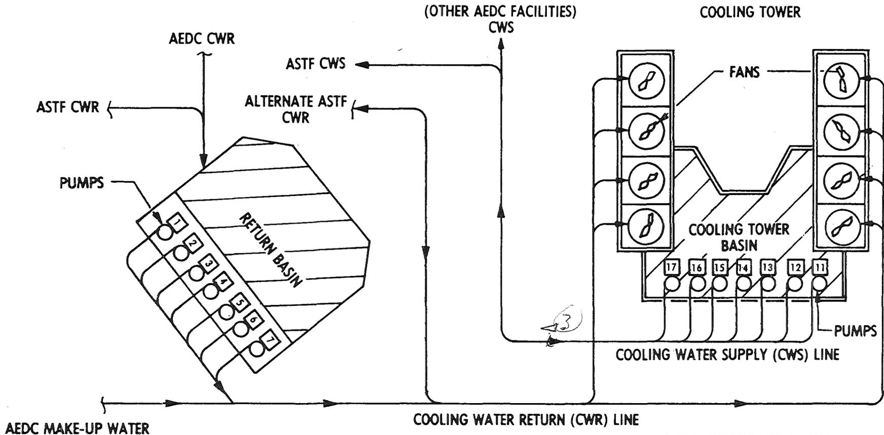
Figure 26. Cooling Tower System Schematic, Closed Loop.
