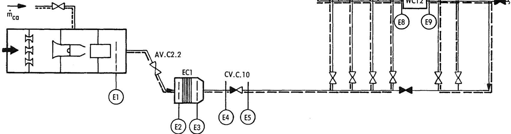
Figure 42. Exhaust System Configuration for Test Scenario No.2.
