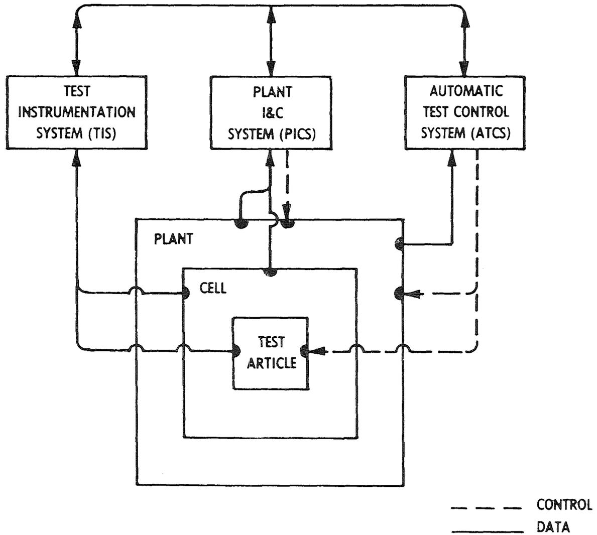
Figure 21. ASTF Instrumentation and Control Interface Diagram.
