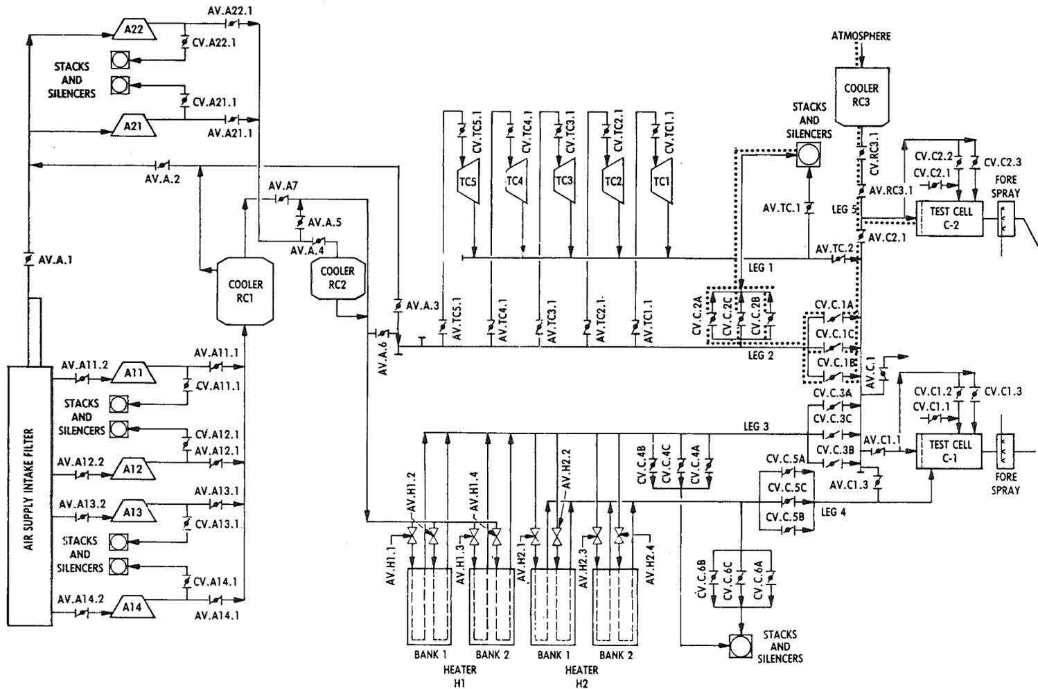
Figure 30. Atmospheric Intake (only) Configuration.
