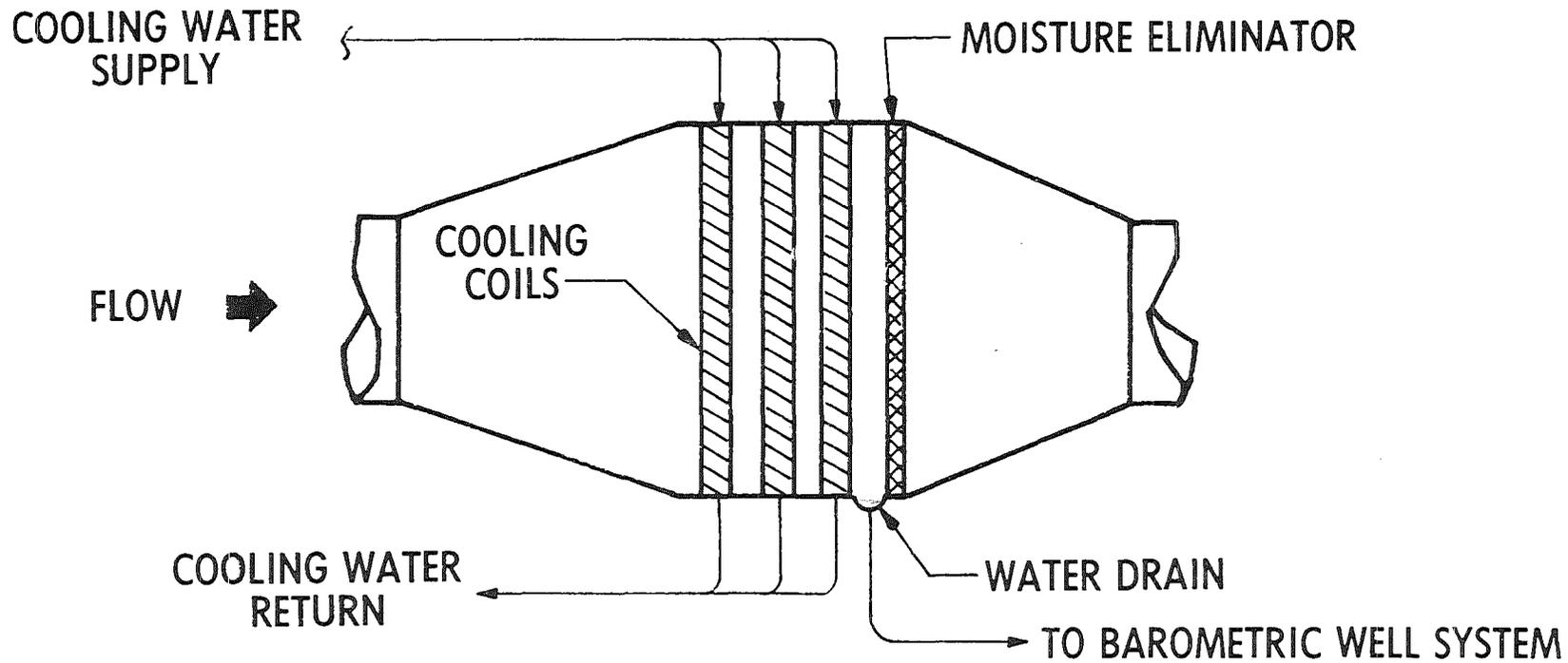
Figure 19. Exhaust Gas Intercooler Schematic.
