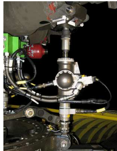
(b) IBC actuator installed on UH-60A rotor.
