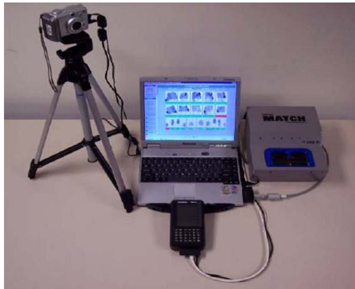
Figure 5. BAT principal components are as follows: digital camera, Toughbook computer, fingerprint reader, and iris scanner.
