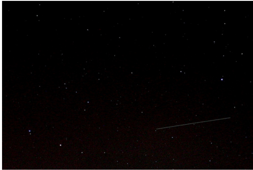
Fig. 9. A satellite streak amongst a field of stars acquired in staring mode (sidereal track) mode of observing. If observed by two telescopes this streak will yield a classical terrestrial parallax determination if position along the streak can be referenced in time.
