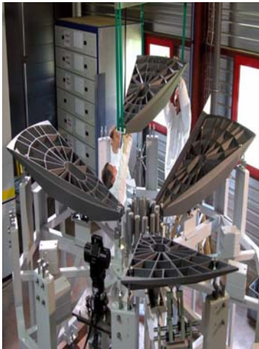
Fig. 6 Herschel Space Telescope--All SiC infrared telescope 3500 mm aperture [7].
