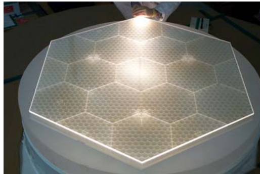
Fig. 3. Kodak’s lightweighted glass mirror segment with ULE honeycomb core produced in the AMSD program. (1.4 m)
