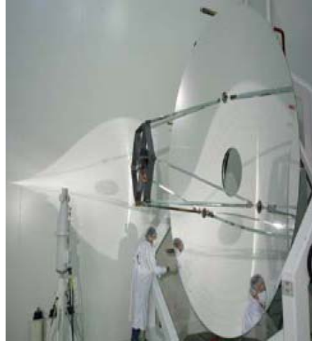
Fig. 6 Herschel Space Telescope--All SiC infrared telescope 3500 mm aperture [7].
