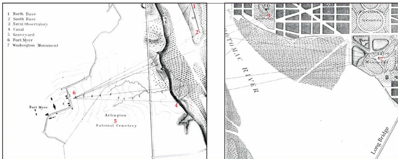
Figure 5. The locations of the temporary observatory and reflectors used by Simon Newcomb and Albert Michelson during velocity-of-light experiments in Washington, DC. The map also shows the triangulation network used by the Coast and Geodetic Survey to measure distances from the rotating mirror (illustrated in figure 4) at Fort Myer to the reflectors at the Naval Observatory (2550.95 meters) and the Washington Monument (3721.21 meters). The experiments were done before the marshlands along the Potomac River were filled and before the Jefferson and Lincoln memorials were built. (Courtesy of the US Naval Observatory.)
