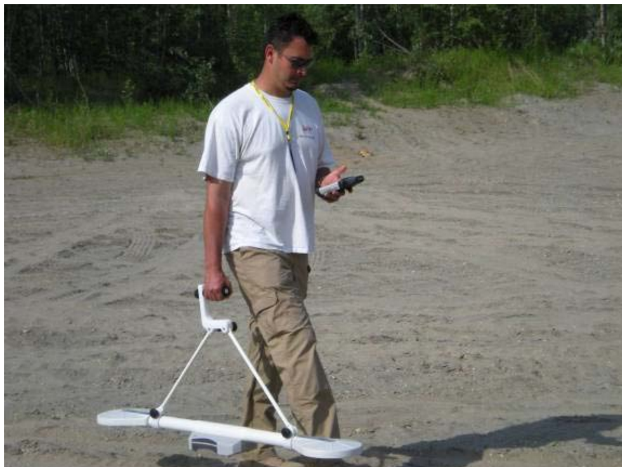
Figure 6. GSSI Profiler EMP-400 electromagnetic induction system.
