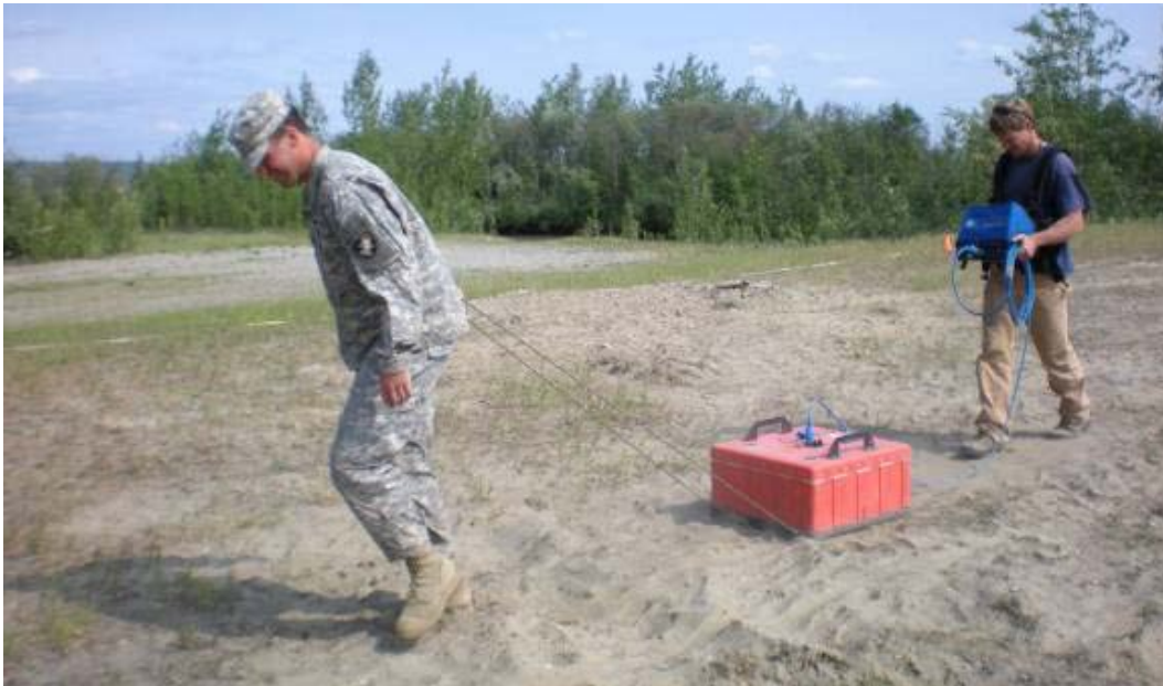
Figure 1. GSSI SIR-3000 GPR with 200 MHz antenna.
