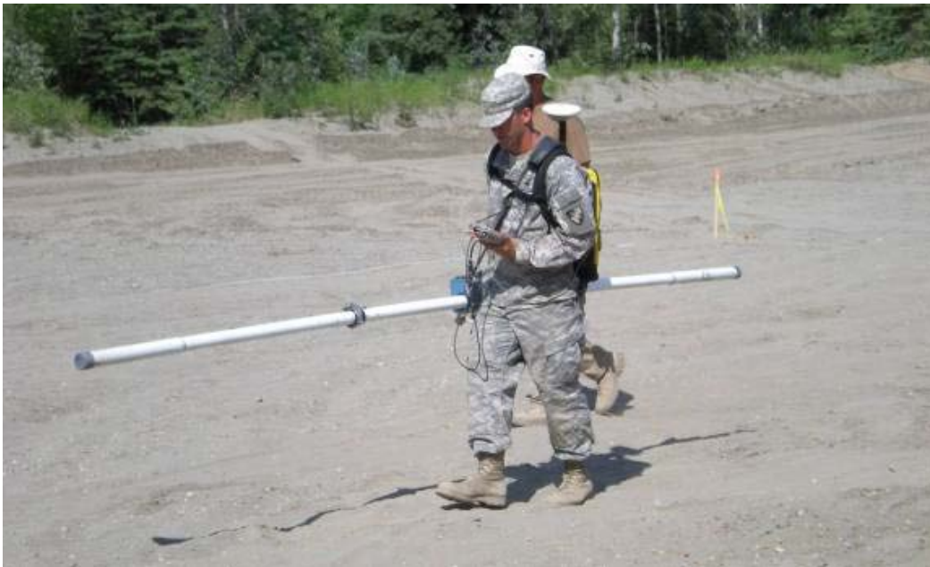
Figure 5. Geonics EM31 electromagnetic conductivity system.
