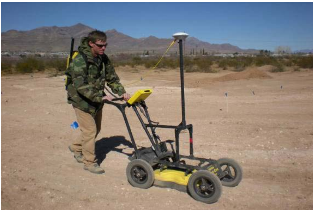
Figure 2. Sensors and Software Noggin Plus GPR with 250 MHz antenna.
