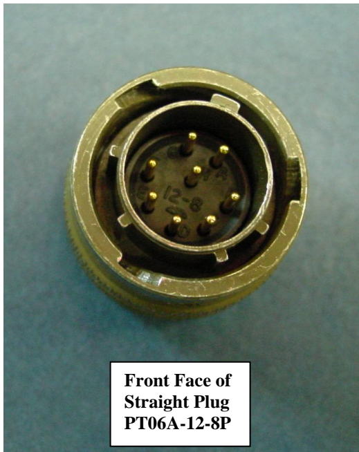
Figure A-6. (Left) Front face and (right) rear face of the Straight Plug PT06A-12-8P.
