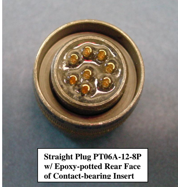
Figure A-7. Straight Plug PT06A-12-8P showing the epoxy-potted rear face of the contact-bearing insert.
