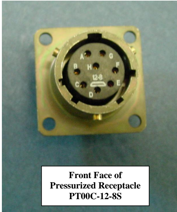
Figure A-5. (Left) Front face and (right) rear face of the Pressurized Receptacle PT00C-12-8S.
