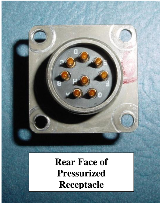
Figure A-5. (Left) Front face and (right) rear face of the Pressurized Receptacle PT00C-12-8S.
