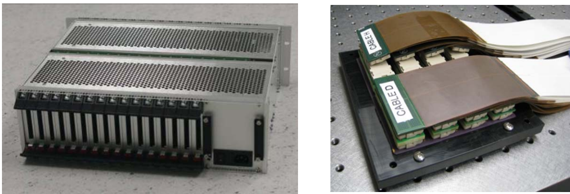
Fig. 4: 4K MEMS DM drive electronics unit (right) designed for the MEMS DMs. The modular design can be configured to drive DMs with 128-4092 actuators and can drive multiple DMs if needed. High-density flex cables connect directly to the back of the DM carrier to minimize its size (right)
