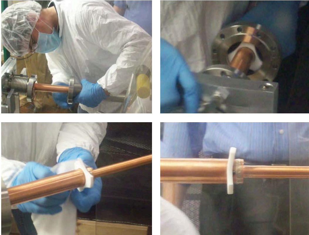
Figure 48. Top left is the initial onset of the binding of the spider. Top right is a close-up of the spider as technicians attempt to slide the surrogate beam tube off the cathode assembly. Bottom left is a picture of technicians cleaning the spider as it will be inserted into the cryomodule along with the cathode assembly. Bottom right shows the deformation of the spider after it was removed from the surrogate beam tube.
