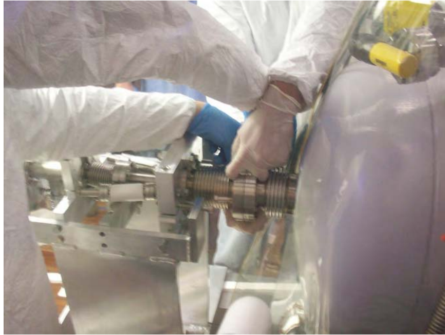
Figure 52. The cathode assembly is mated to the cavity and a vacuum tight connection is made. The cavity was then placed back under vacuum.
