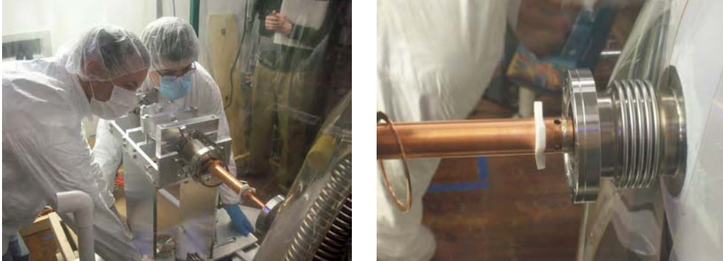
Figure 50. On the left, technicians begin to move the cathode assembly into the cavity. On the right, the teflon spider, due to deformation, now no longer has clearance inside the beam tube to easily slide without contact. In this photo, we can see that after pulling the cathode assembly back out slightly, the spider has slid along the assembly from its intended position (where the holes are visible).
