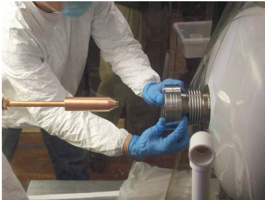
Figure 49. The last seal before opening the cavity beam tube is broken to insert the cathode assembly. Note the niobium cathode button is visible at the tip of the cathode assembly.
