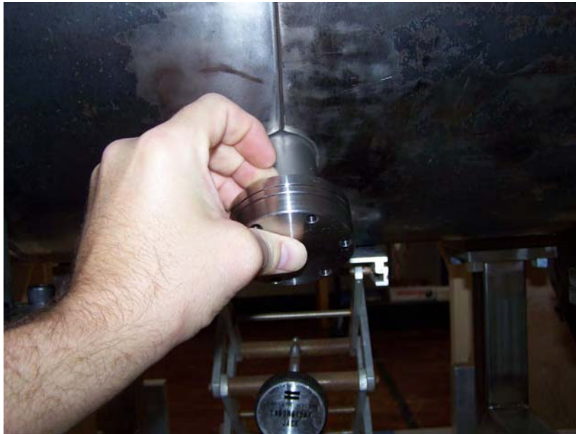
Figure 39. When the cavity is warm, it rests upon two “shipping feet” that support the cavity in addition to the liquid helium fill tube and exit beam tube. When cold, the contraction of these tubes lifts the cavity from these supports, isolating it thermally and mechanically.
