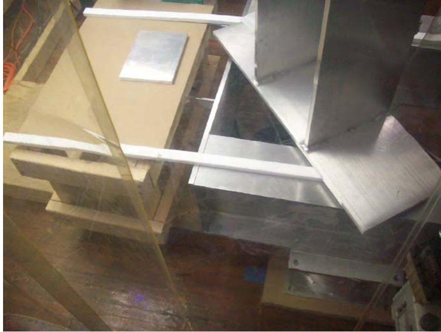
Figure 46. Two thin teflon rails are used to minimize friction when sliding the cathode assembly structure into place. The step behind the foundation is to allow the structure to slide behind the cryomodule with room for the cathode to clear the beam tube prior to insertion. One of the aluminum pads for mounting the structure to the foundation can be seen near the top of the photo, between the rails.
