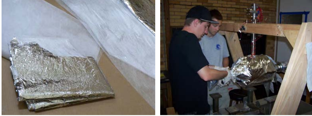
Figure 34. Insulating blanket material (shown on left) is wrapped around the helium vessel.
