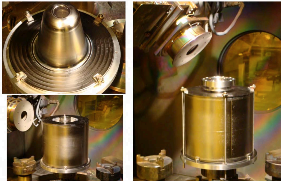
Figure 28. The NPS cavity in the electron beam welder at Sciaky, Inc. Top left is the nose cone being welded to the base plate. Bottom left is the base plate being welded to the outer conductor of the cavity. The photo on the right is a conflat flange being welded to the anode side of the cavity.
