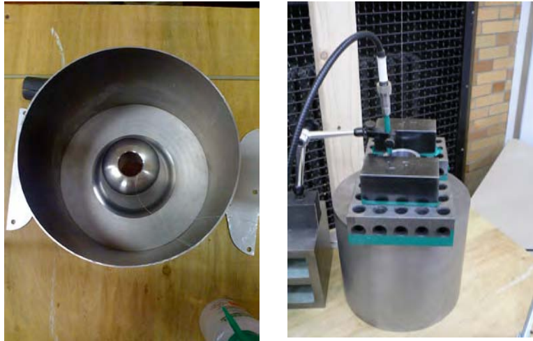
Figure 94. NPS gun/booster cavity configuration for eigenfrequency testing. On the left, is the cavity with the output end removed to see the nose cone. On the right, we see the cavity as tested. The blocks on top are there to provide weight to make good electrical contact with the sides of the cavity.
