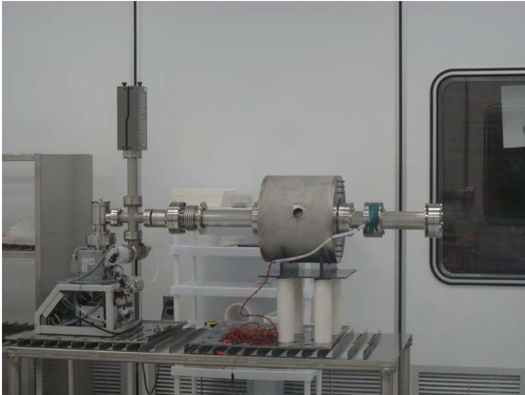
Figure 31. The NPS SRF cavity in the class-100 clean room after chemical processing and high-pressure rinse. The cavity is under vacuum to remove the remaining water and to verify the cavity is still vacuum tight. Note that the beam tubes have also been attached to the cavity in preparation for the next stage of assembly.
