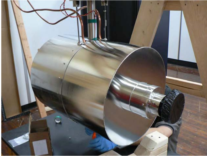
Figure 36. MuMetal shield installed around the liquid nitrogen shield. Note that superconducting solenoid is encapsulated by MuMetal. The black covering indicates this picture was taken during test fitting.
