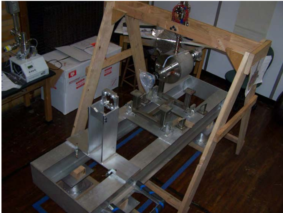
Figure 33. The cavity is in place and aligned to the support foundation.
