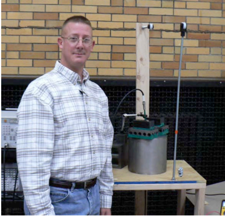
Figure 96. LCDR Sean Niles stands next to the measurement system for the cavity bead pull. A transmitting antenna is inserted from the top of the cavity and a receiver below. The pulleys are connected via thin fishing line and attached on one end to an electric motor and a weight on the other to keep the line taught and to provide a reference point for linear position measurements.
