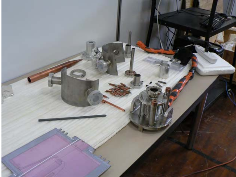
Figure 38. The conning tower assembly prior to assembly and mating to the vacuum vessel.
