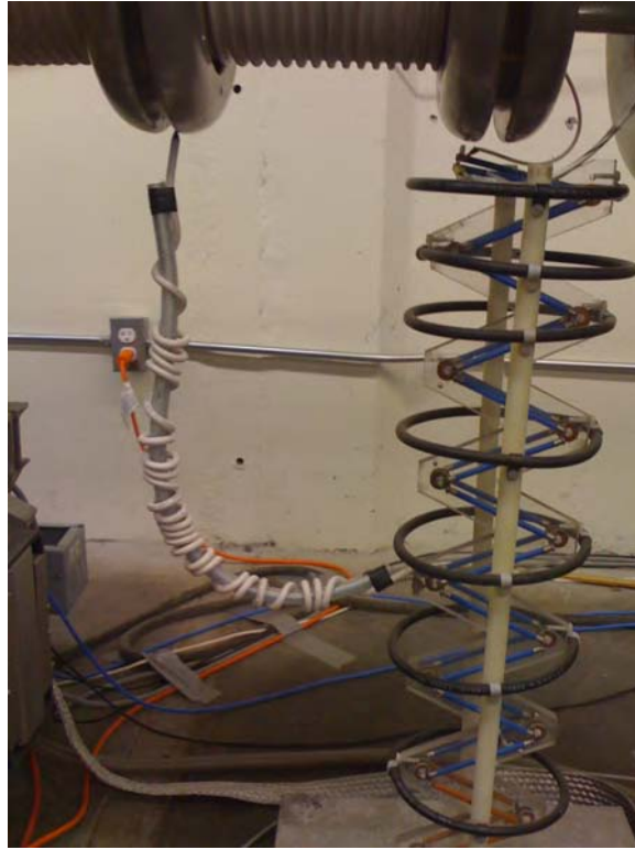
Figure 61. The DC gun voltage divider showing the resistive ladder on the right connecting ground to the cathode potential. The white wire coming off to the left is an adjustable connection to the focusing electrode.
