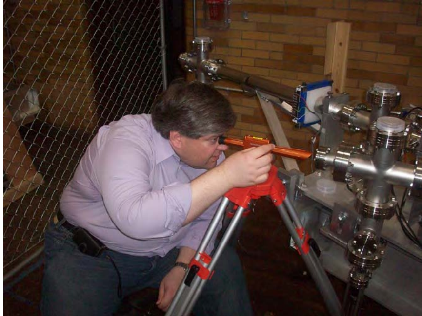
Figure 53. Dr. John Lewellen observes the positioning of the cathode assembly relative to the cavity nose cone using an optical transit.
