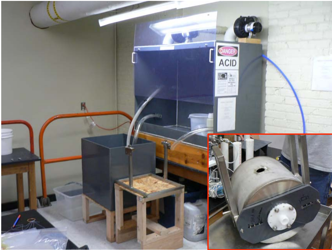
Figure 29. This station was used for performing the buffered chemical polish of the NPS cavity. In the inset at lower right is the cavity placed in the rocking cradle that mates with the stand shown just to the right of the cooling tub. The hole shown in the inset is the connection to the liquid helium fill tube and leads to the exterior of the niobium cavity.
