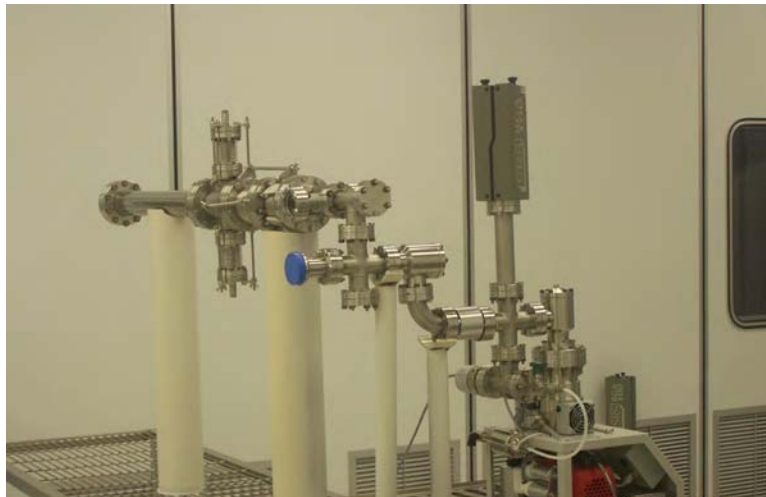
Figure 40. The coupler was maintained in a clean environment, under vacuum, while the cryomodule was assembled. The coupler is shown on the left. The vacuum pumping stand is on the right.
