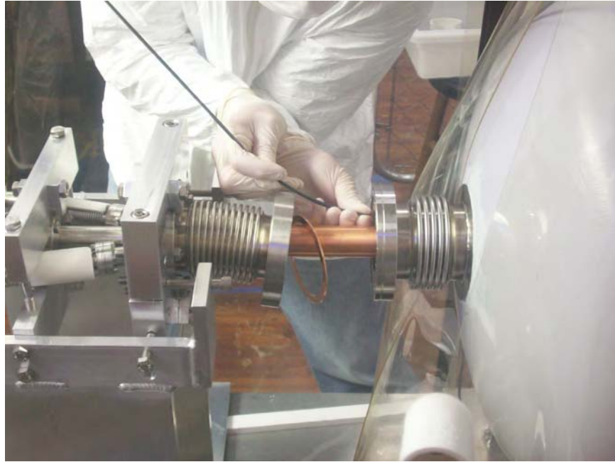
Figure 51. A PVC pusher is used to position the spider during insertion.
