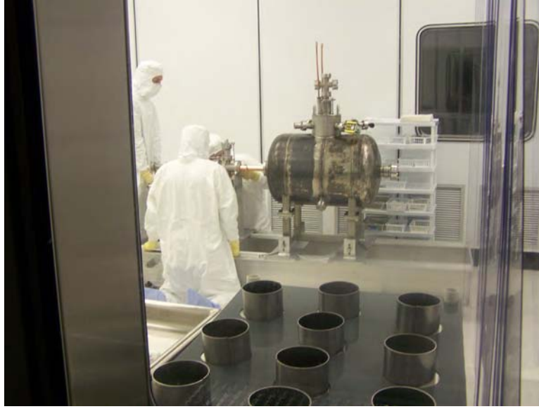
Figure 42. Insertion of the RF coupler into the cryomodule beam tube.
