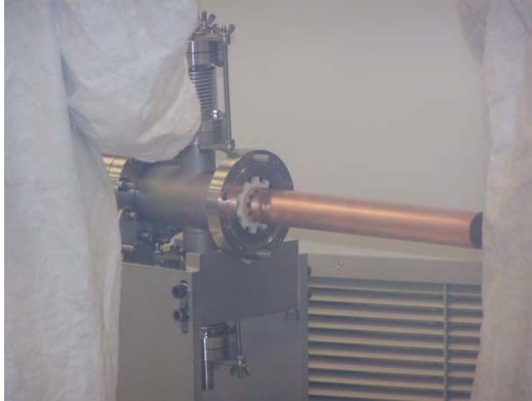
Figure 41. The RF coupler assembly with surrogate beam tube removed. The tube is supported at the visible flange by a teflon spider.
