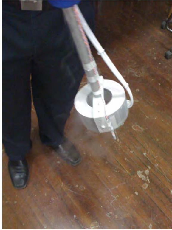
Figure 103. Inspecting the superconducting solenoid after removal from the liquid helium bath.
