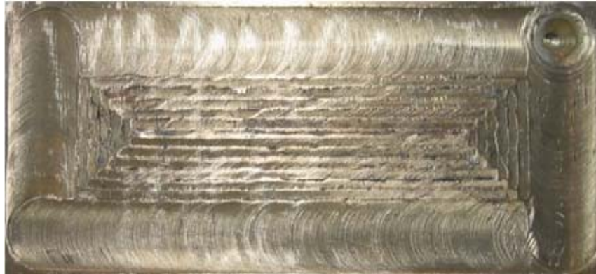
Figure 9. Example of a rectangular spiral pattern used for FSP of multiple pass plates. From [4]
