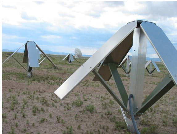
Fig. 3.— Photo of several LWDA elements showing the droopy blades and an NRAO VLA antenna in the background.
