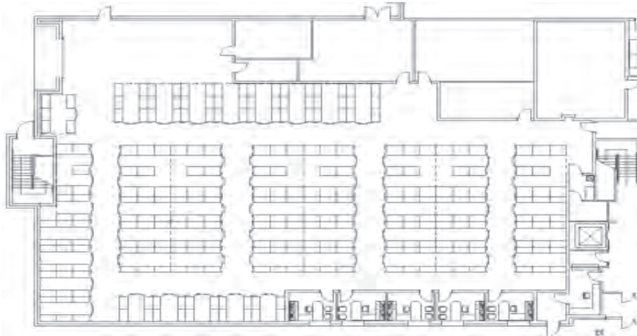
Figure 4-21 Unit Storage with Staging and Supply Office
