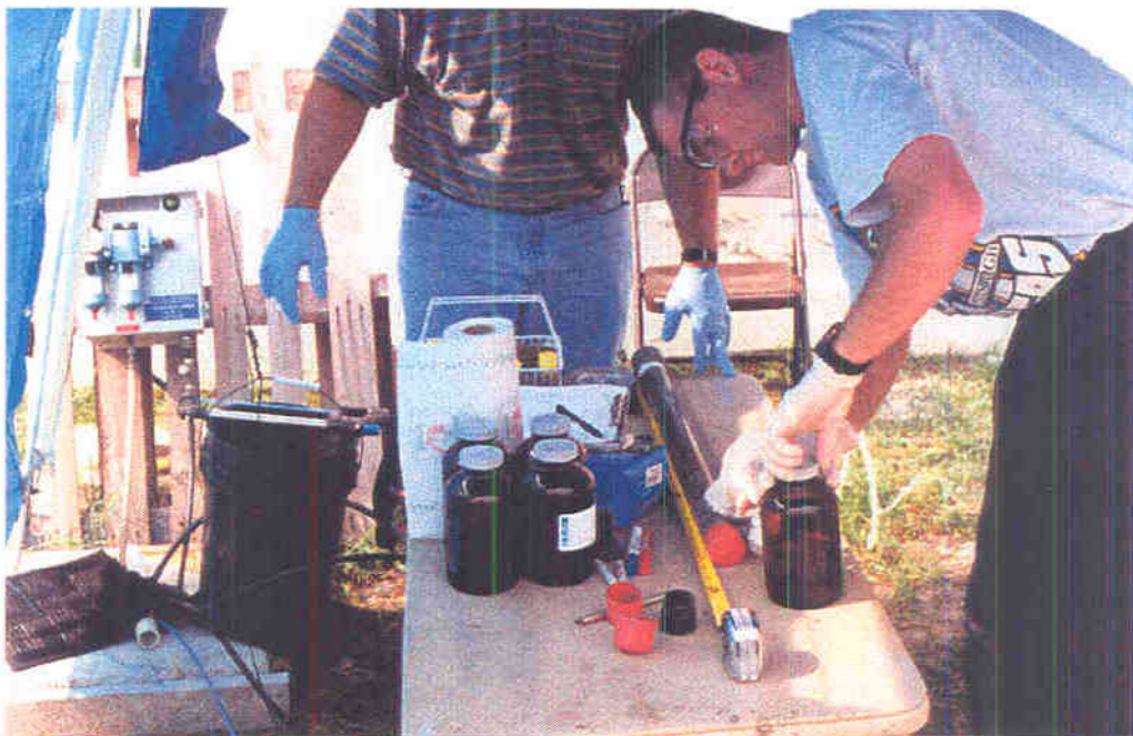
Preparation of sample jar with methanol for in-field presentation of soil samples
