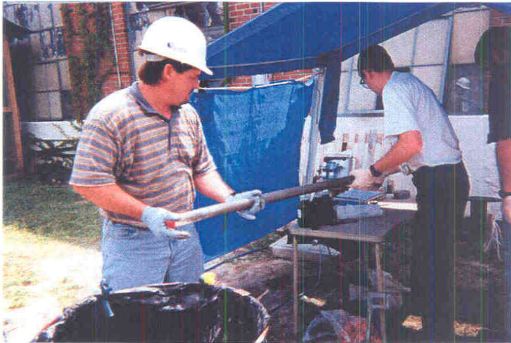
Recovered soil core in a sample tube liner
