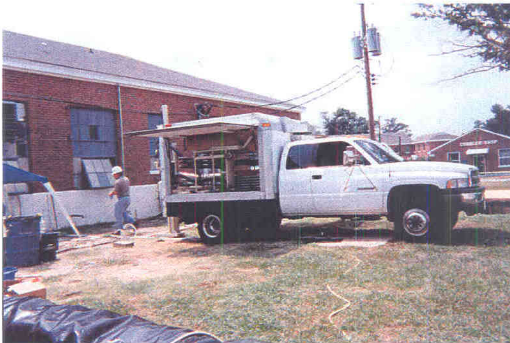
The EPA truck-mounted Geoprobe used for post-SEAR (final) soil sampling
