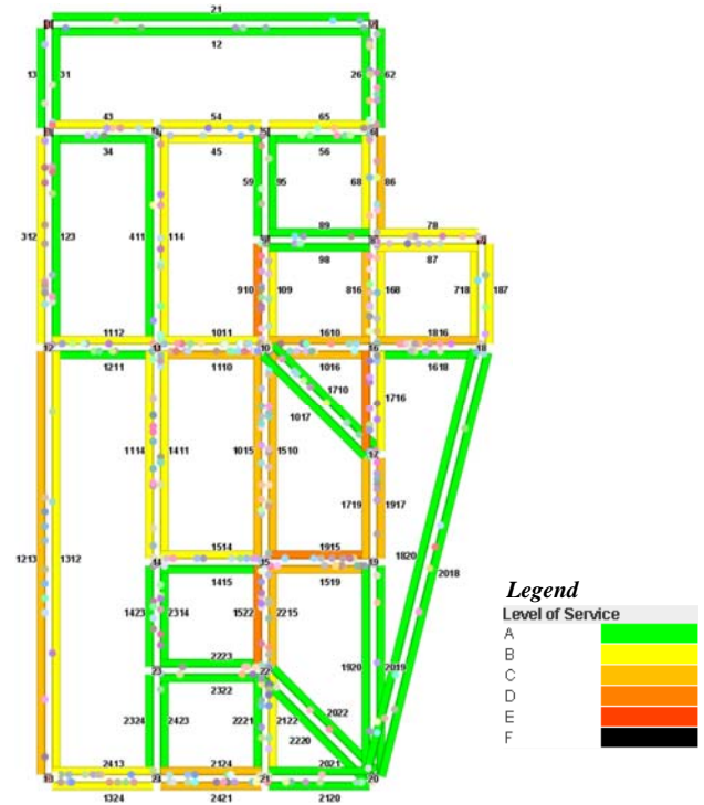
Figure 33 Traffic congestion (volume-capacity ratio) by the DTA model (night scenario)
