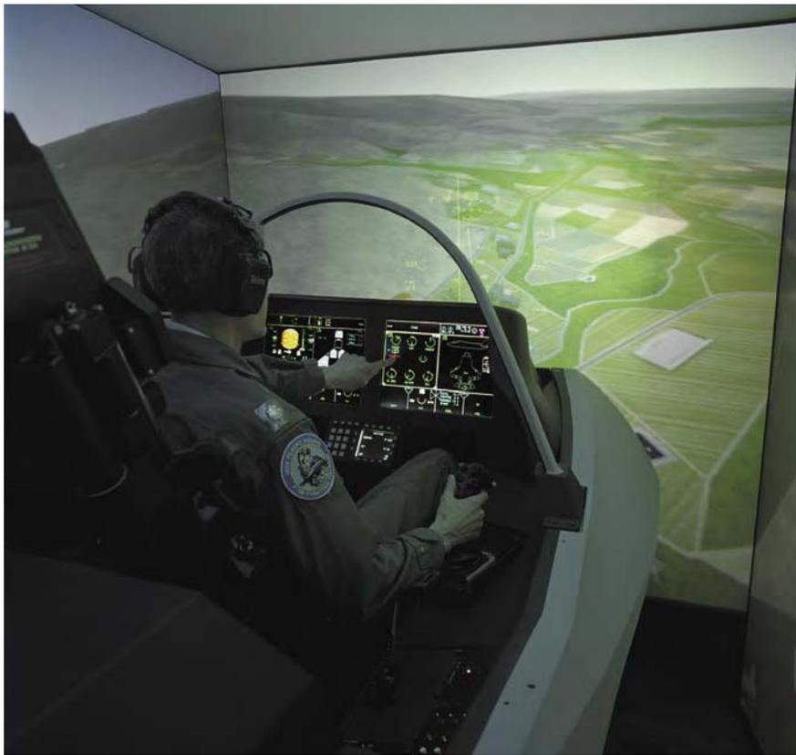
Photo of a high-fidelity cockpit used in Lockheed Martin's Manned Tactical Simulator
