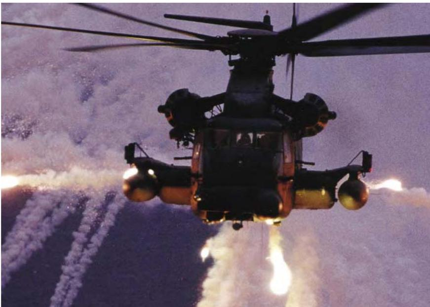
Photo of a MH-53J Pave Low helicopter dispensing flares.
