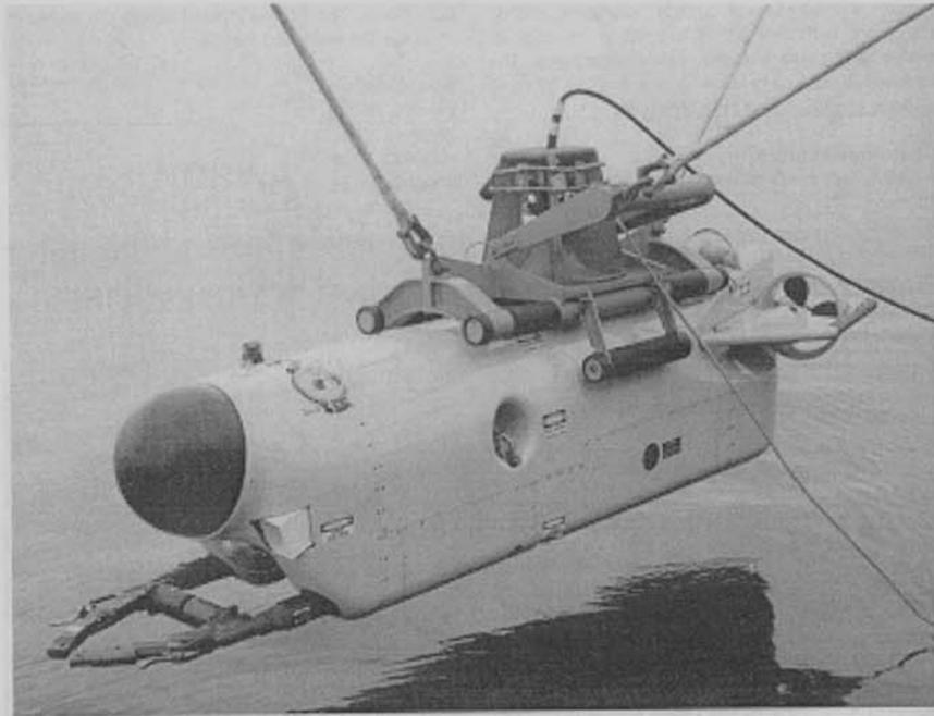
MNS vehicle showing handling arrangement
