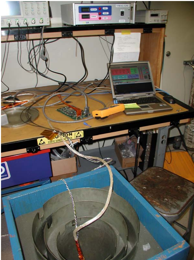
Figure 15. GSE control box (top of image), PC (middle), and shield cans (bottom). Figure 14 is looking down into the shield cans. Next to the PC and multi-meter on the bench is the engineering electronics unit.
