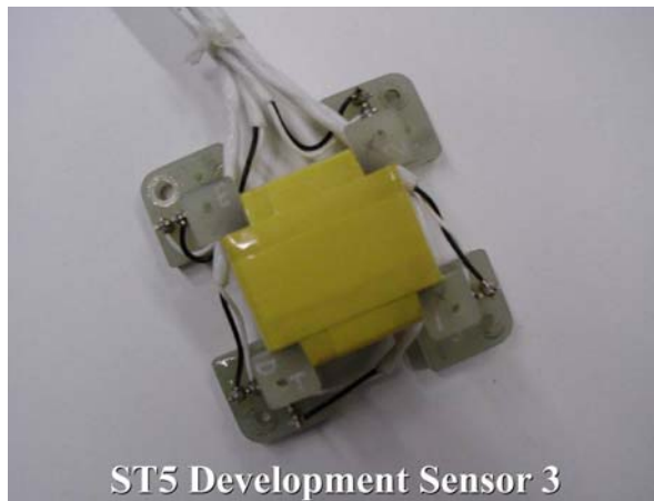
Figure 6. The 3-axis ring-core fluxgate sensor fabricated by UCLA for ST5. A similar design is used for DSX. The DSX sensor occupies a volume of 5x5x5 cm.
