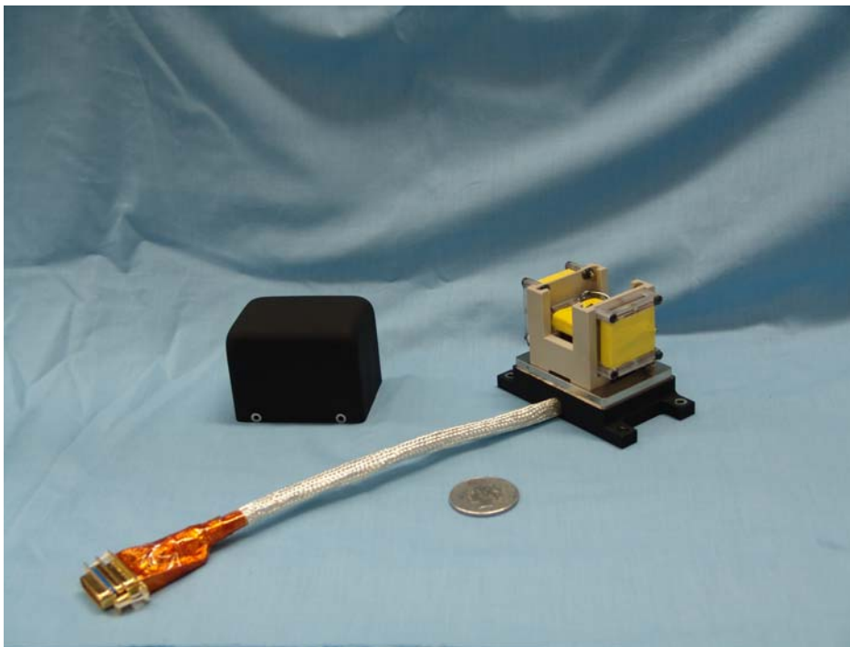
Figure 13. The Flight sensor, chassis and a US quarter for scale.
