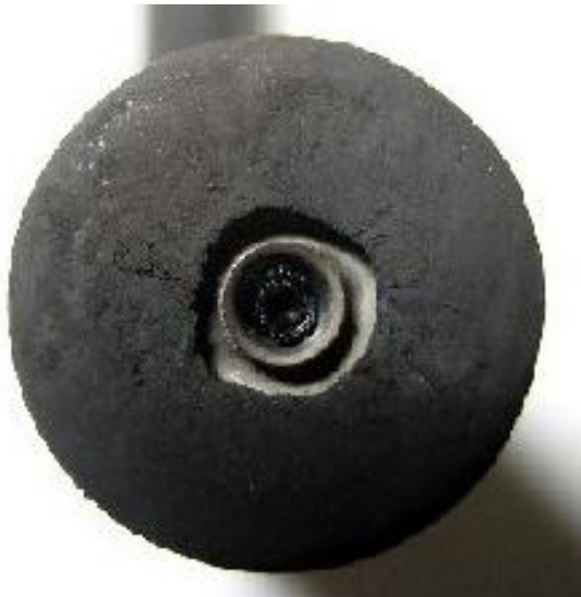
Figure L-3. Laughlin J85 Fuel Spray Nozzle After 1,350 FH
