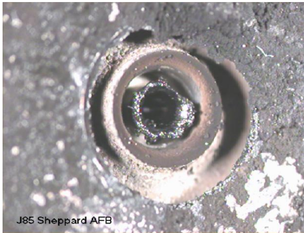
Figure 6. Coking Around Primary Fuel Nozzle, J85 Engine
