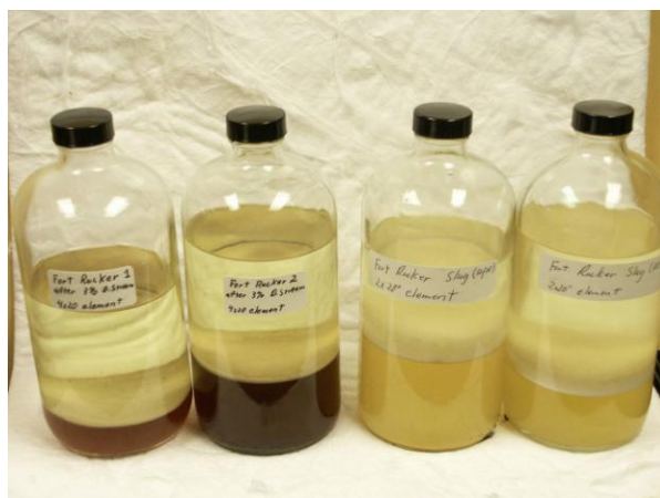
Figure 26. “Goo” Found in Filter Element Vessel
