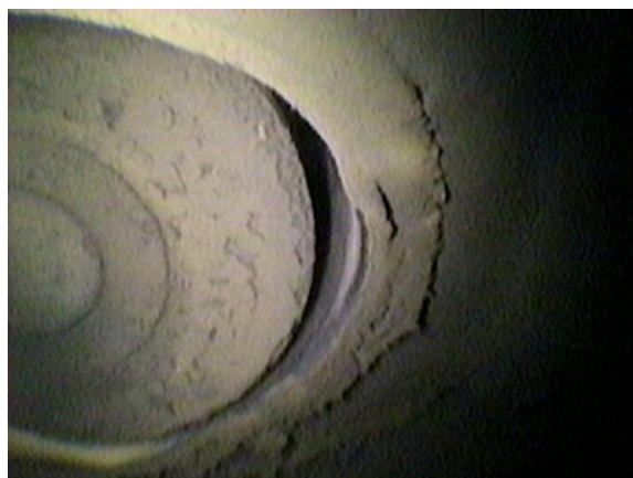
Figure 88. Baseline Condition of Ignitor
