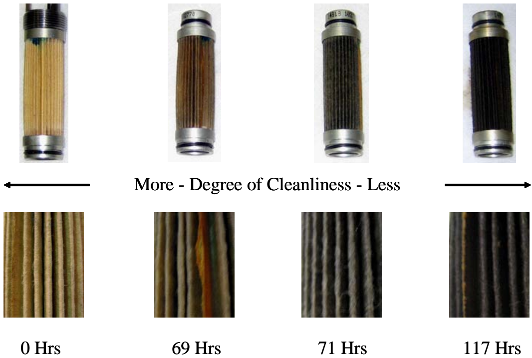
Figure L-18. J69 Fuel Control Filter Condition after Using JP-8
