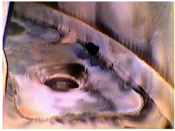
Figure 64. T700 Engine Combustor Dome, EOT: 1722; +100 Time: 395 Hrs.
