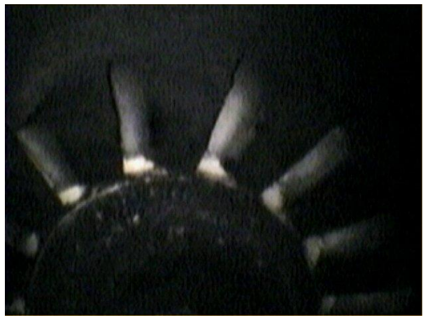
Figure 34. T64 Combustor Nozzle Cup, EOT: 857 FH; +100 Time: 815 FH
