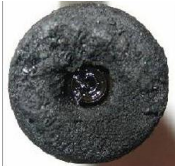
Figure L-4. Comparison Unit J85 Fuel Spray Nozzle After 200 FH
