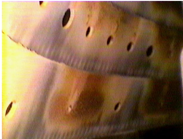
Figure 75. T700 Engine Combustor Wall, EOT: 2495; +100 Time: 344 Hrs.
