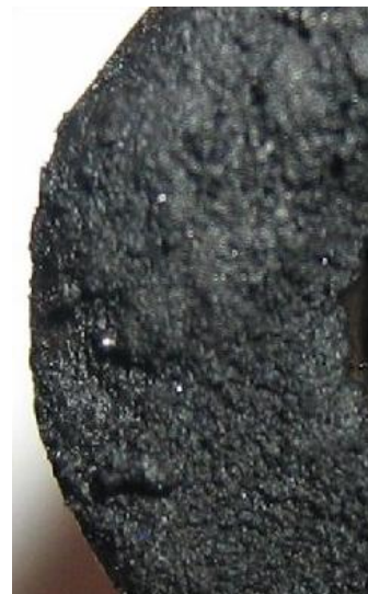
Figure L-6. Magnified Carbon Deposits From JP-8 Use
