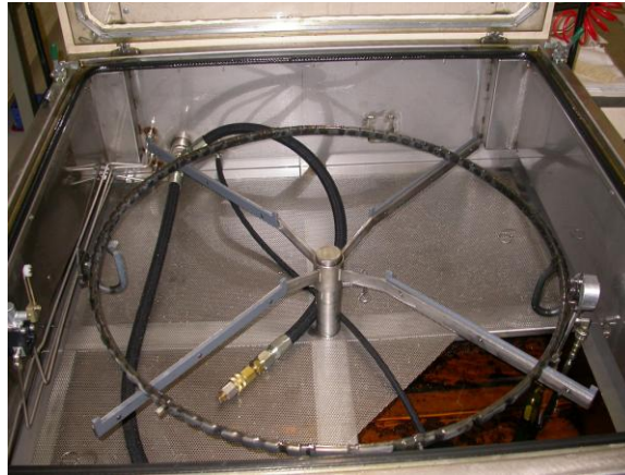
Figure 91. Augmentor Spray Ring Flow Bench Showing Spray Ring Mounted
