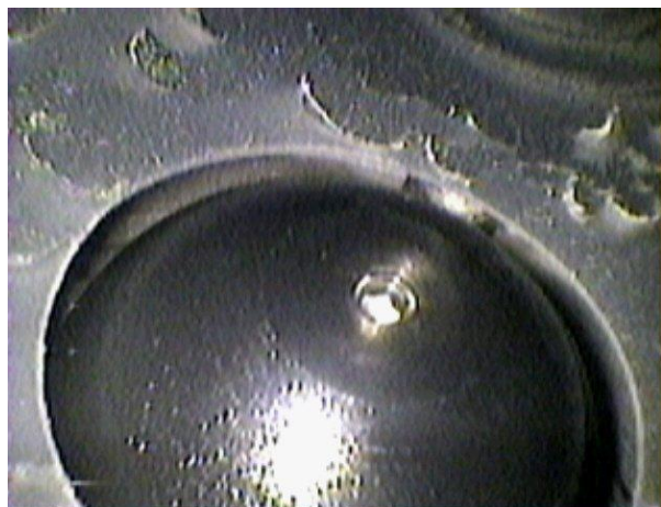
Figure 42. MH-53 Heater Combustor Nozzle, +100 Time: 179 Hrs
