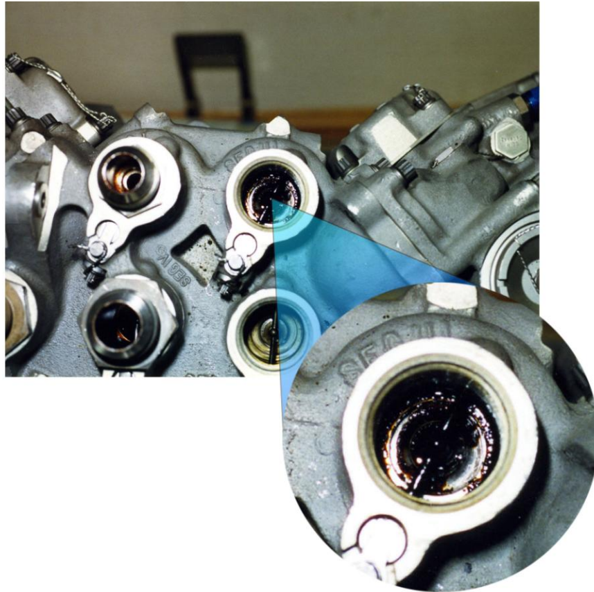
Figure 15. Coke in AFC SEG III Fuel Outlet Port
