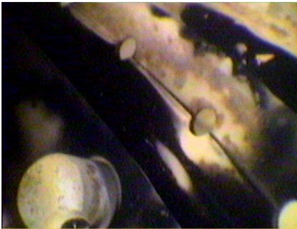
Figure 49. T400 Engine Fuel Nozzle Shroud, Hours Since Overhaul: 1215
