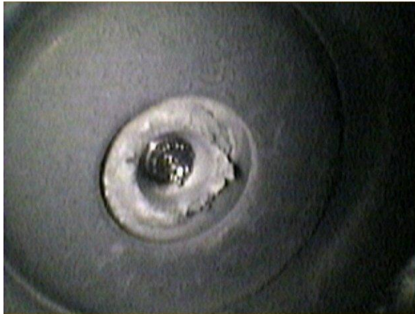
Figure 35. T64 Combustor Nozzle, EOT: 103 FH; +100 Time: 61 FH
