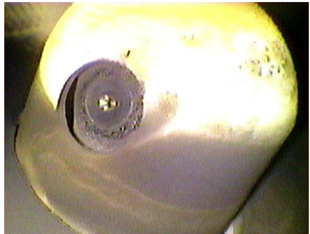
Figure 50. T400 Engine Fuel Nozzle, Hours Since Overhaul: 1215
