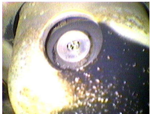
Figure 46. T400 Engine Fuel Nozzle, Hours Since Overhaul: 109
