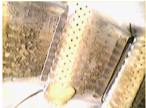
Figure 38. T64 Vane, EOT: 857 FH; +100 Time: 815 FH
