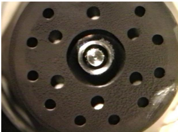
Figure 89. Carbon Deposition on Nozzle Face After Using Jet A+100
