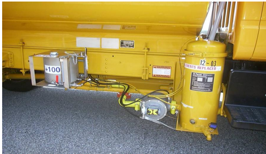
Figure 22. Additive Reservoir Tank and Injector
