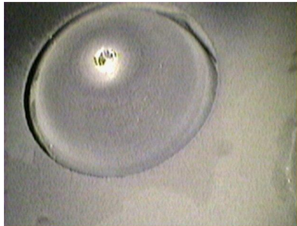
Figure 40. MH-53 Heater Combustor Fuel Nozzle, +100 Time: 0 Hrs
