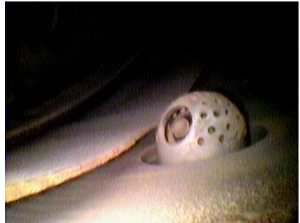
Figure 68. T700 Engine Primer Nozzle, EOT: 1722; +100 Time: 395 Hrs.
