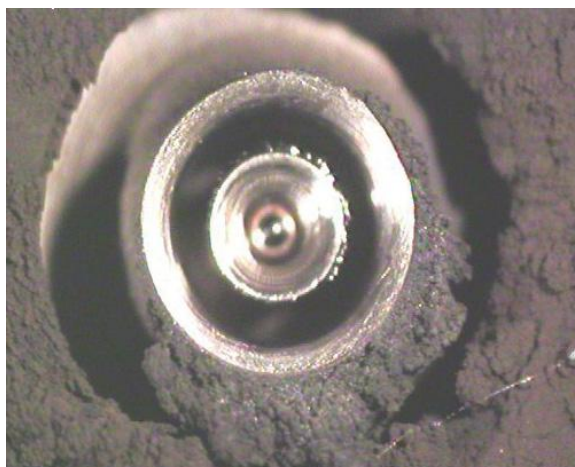
Figure 84. Coke Deposits Around Primary Fuel Nozzle
