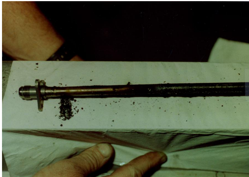
Figure 11. Coke on ASEP Inner Tube
