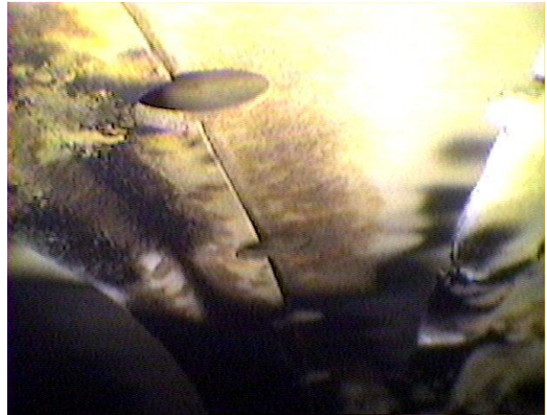
Figure 48. T400 Engine Combustor Wall, Hours Since Overhaul: 1215
