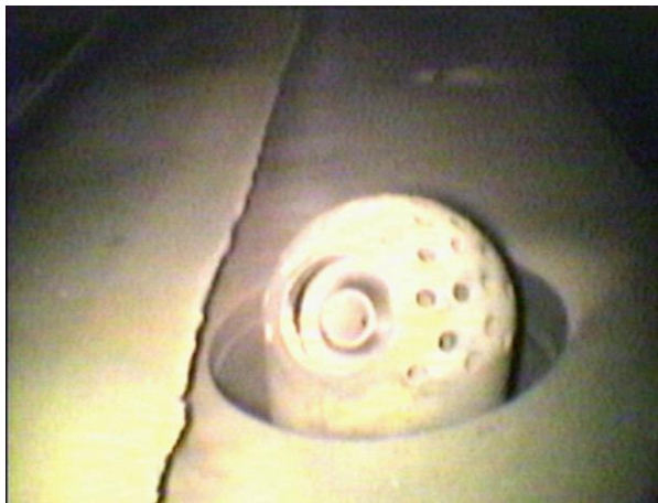
Figure 63. T700 Engine Primer Nozzle, EOT: 1327; +100 Time: 0 Hrs.
