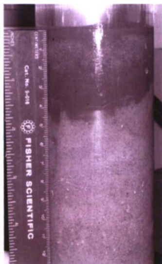
Fig. 7. Photograph of core FWB9-2 taken in conjunction with IMP2 run 117 at horizontal coordinate 273 cm. This location is marked by the third green circle from the left in Fig. 5. A mud layer occupies the top 4 cm of the core and contains a sand inclusion about 1 cm thick.
