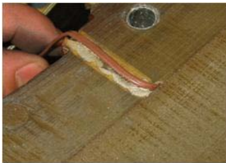
Thermocouples embedded for internal measurements
