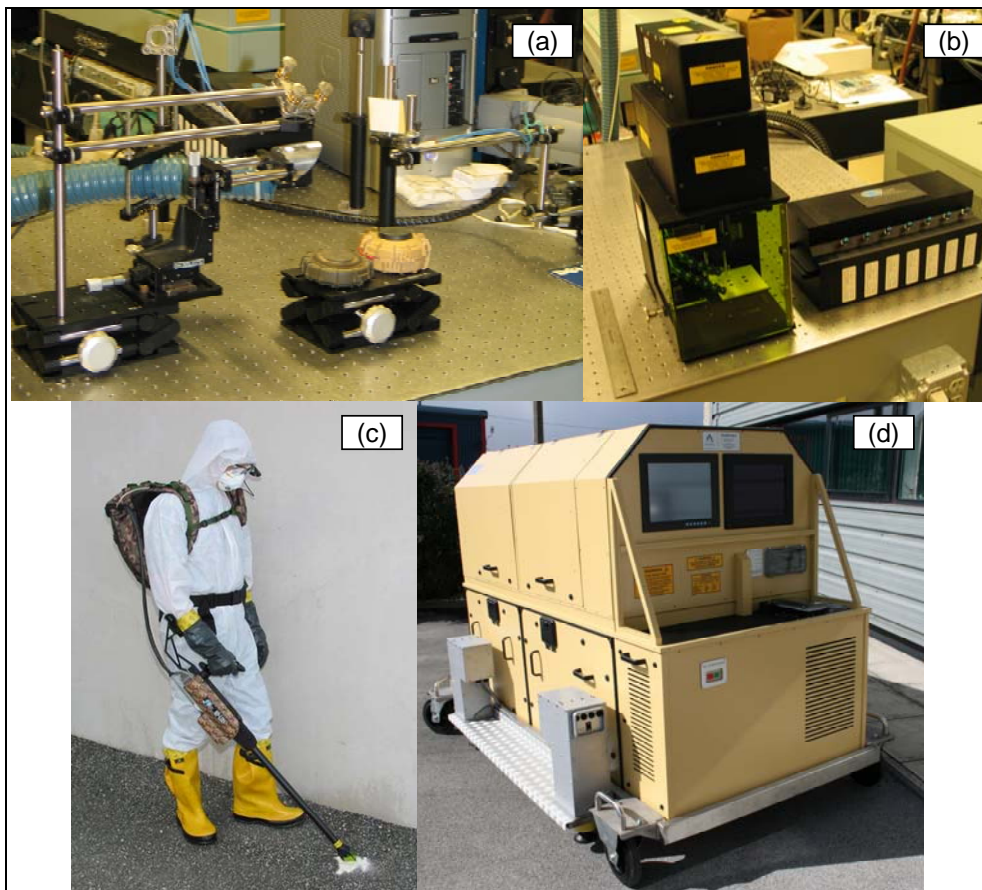
Figure 2. Photographs of ARL LIBS systems: (a) a laboratory LIBS setup, (b) a commercial LIBS system by Ocean Optics, Inc., (c) a prototype man-portable LIBS device, and (d) a prototype standoff LIBS system developed for 100+ m detection and discrimination of explosive residues.
