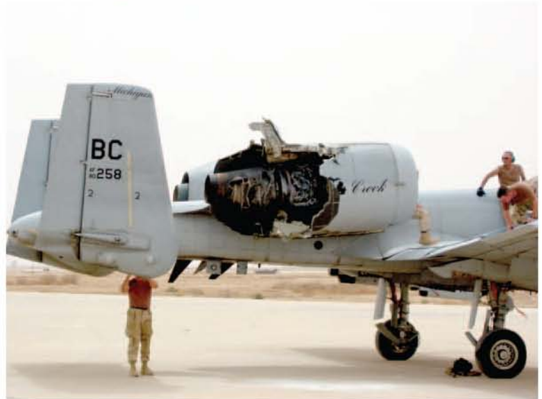
Combat damaged A-10 Warthog
