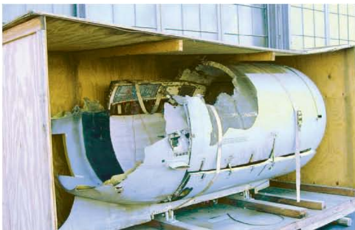
Combat damage engine nacelle
