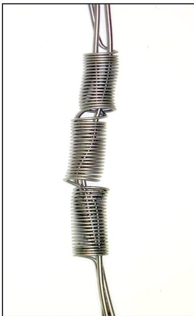
**Figure 2-2. Stacked coil arrangement for feed vaporization**
