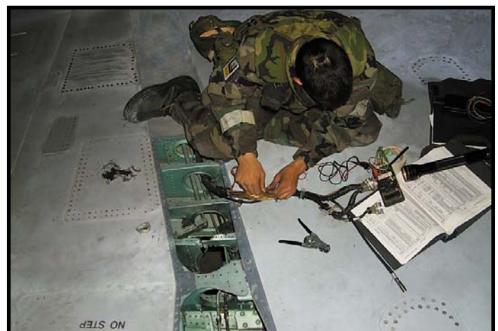
SrA Bobby Lynch troubleshoots a damaged wire bundle during Serene Robins 00-02. Lynch, a member of a 14 person F-15 ABDR team, used a computerized wire program to speed the repairs to the damaged aircraft.
