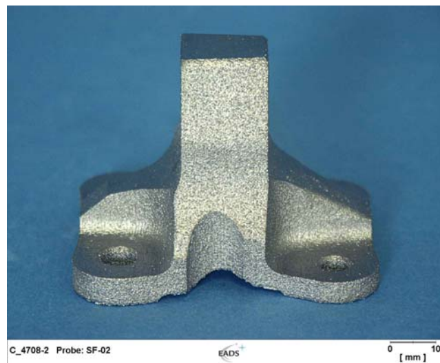
Figure 13: Ti-Al6-V4 demonstrator part manufactured by laser melting in the powder bed.
