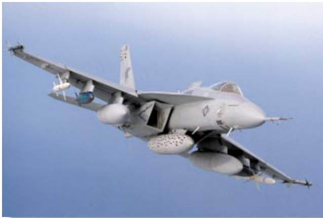
The F/A-19E “Super Hornet” completing its first in-flight tests with ordnance. Official DoD photo by Vernon Pugh.
