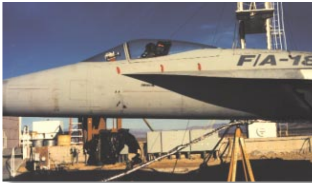
Figure 1. Ullage explosion setup in Tank 1
