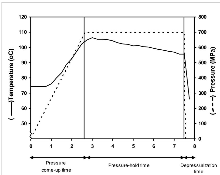
Figure 15. Sample pressure-temperature profile observed during PATP. Data presented are mean values of two independent trails.
