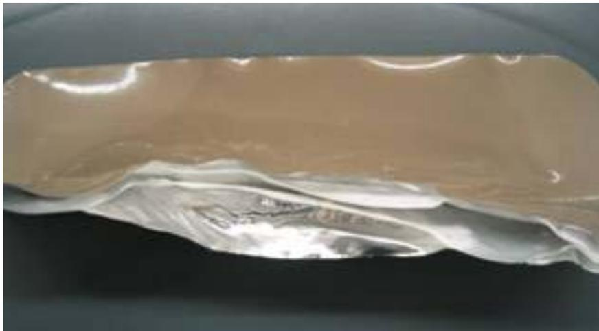
Figure 9. MRE pouch delamination.
