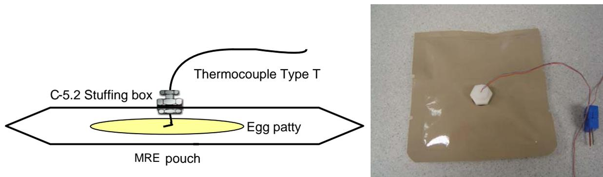
Figure 2: Flexible pouch with attached thermocouple.
