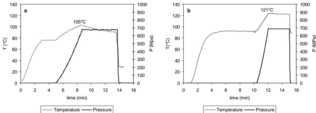
Figure 7. Typical temperature and pressure profiles during HP/TS processing in water/egg patty system at (a) 700MPa/105°C/5min and (b) 700 MPa/121°C/3min.
