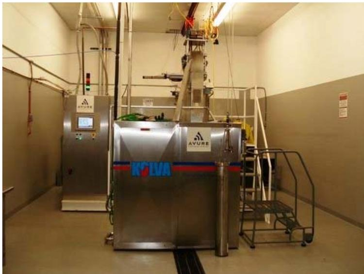
Figure 4: DUST 35L machine (QUINTUS Food Autoclave Type 35L-600 Avure Technologies, Kent, WA, USA) at National Center for Food Safety and Technology.
