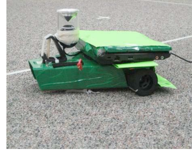
Fig. 38. Stinger robot assembly with serializer, EEE PC and omnidirectional camera
