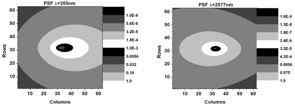
**Figure 1.** Adjacency kernels at 355 nm (left) and 2577 nm (right). The sensor is located to the left of the center in these simulations. Image pixels are 20m x 20m. The aerosol optical depth is 0.067 and the visibility is 100 km. The Rayleigh contribution to the kernel is 84% at left and 5% at right.
