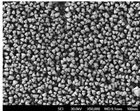
**Fig. 2.** SEM image of W nanorods grown on a glass substrate.
