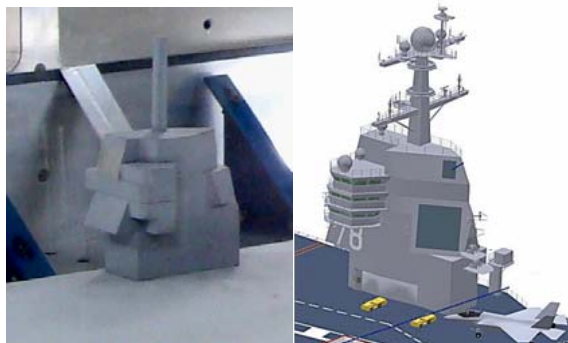
Figure 4. CVN-78 Ford Class Superstructure & Model
