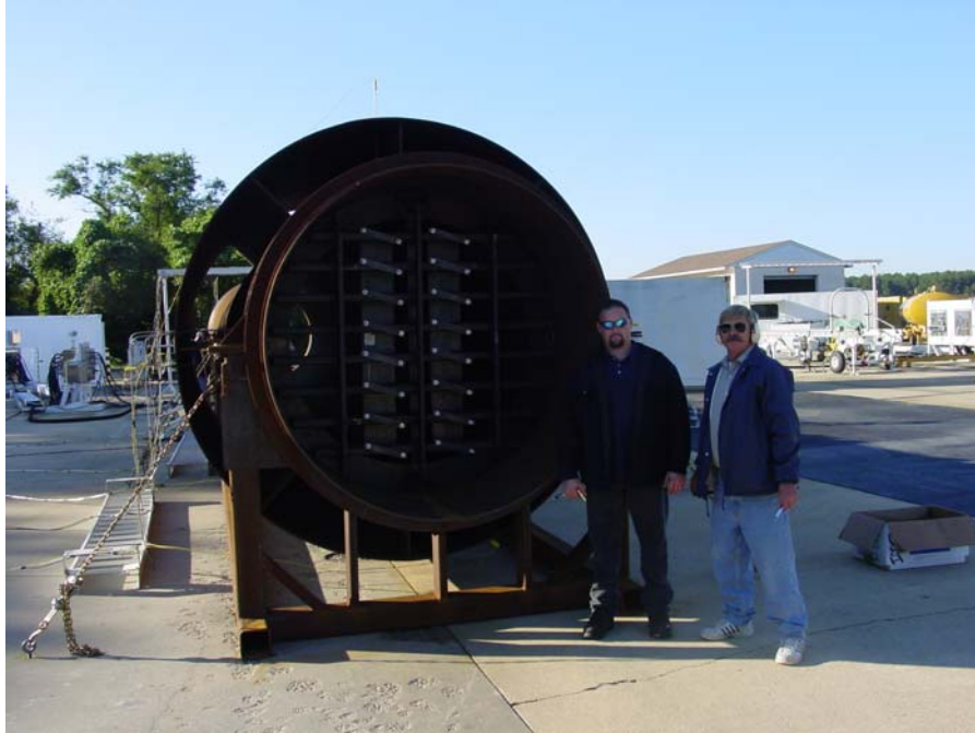
Figure 3.23 A Job Well-Done. After Allowing NAD to Cool From Previous Engine Run, “Plates” Were Installed in \frac{3}{4} Hour Saving Critical Engine Test Time.
