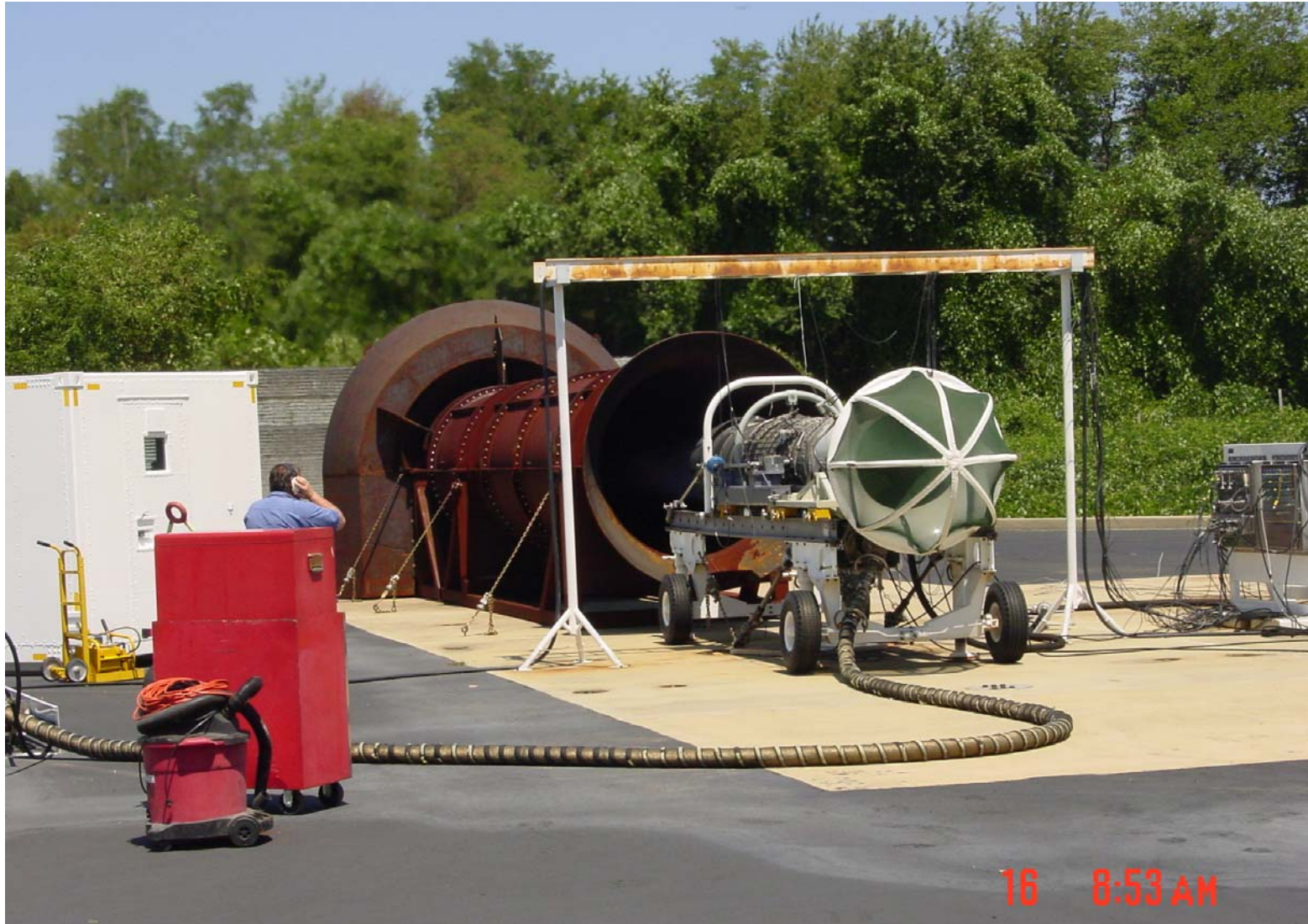
Figure 1.1 NAD installation, Including Flow Deflector, with F-404 Engine.
