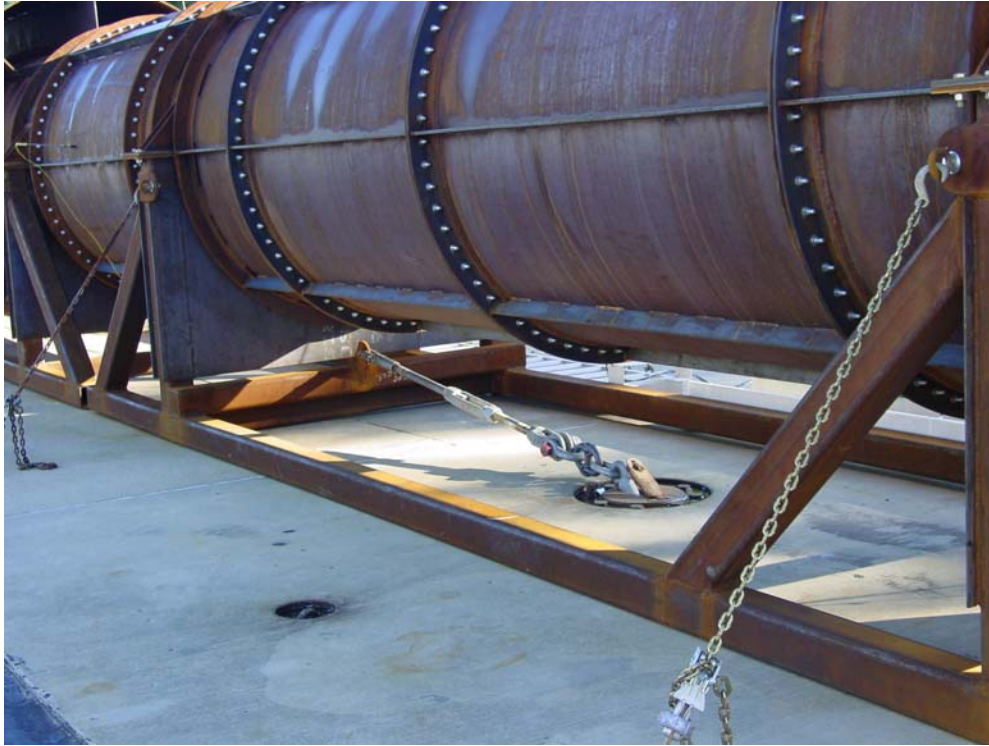
Figure 3.17 View Showing Bolted Sections of NAD, Reinforcing Elements, Thrust Turnbuckle, and Tie-Down Chains.
