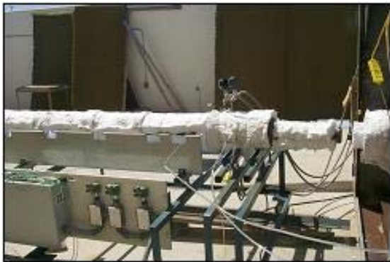
Figure 2.5 Sub-Scale 1-1/2 inch Simulated Engine and AAR for Noise Testing.
