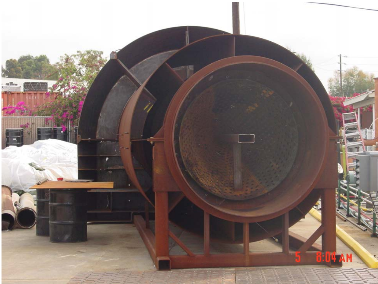
Figure 3.10 Rear View of NAD Assembled With Exhaust Deflector at GE-EER Test Facility.
