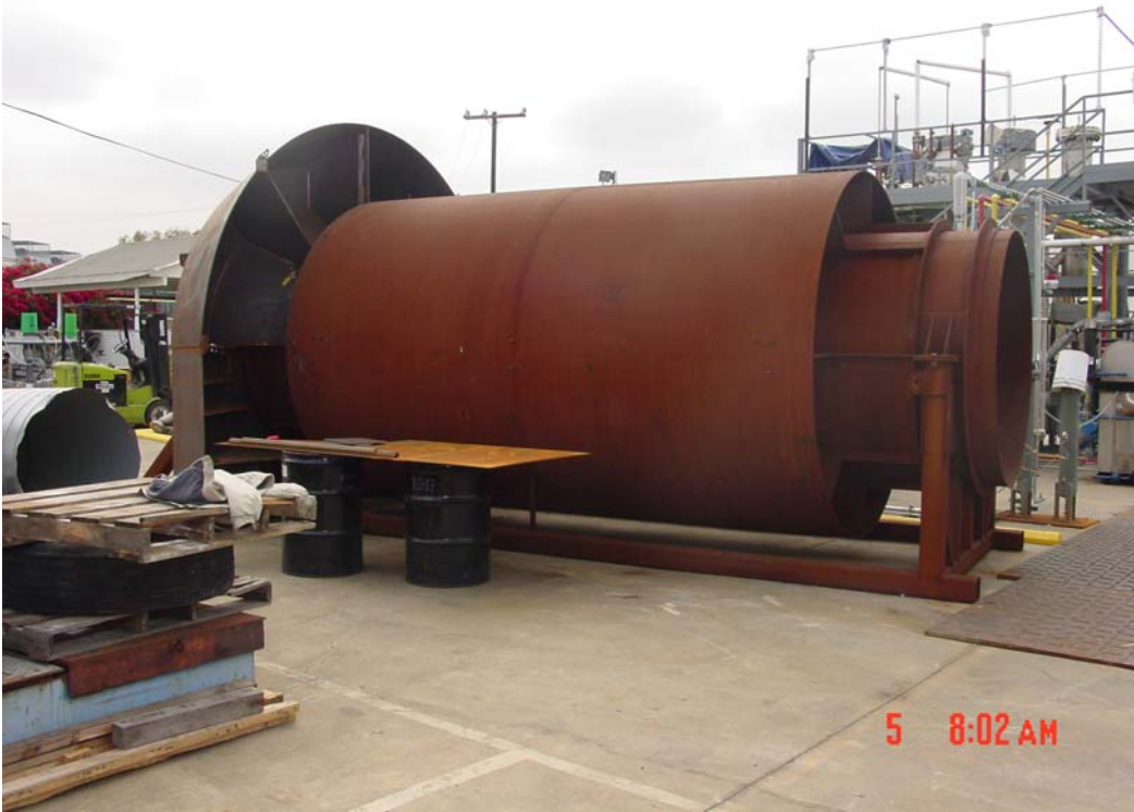
Figure 3.9 Exhaust Deflector Being Trial Assembled With NAD at GE-EER Site.
