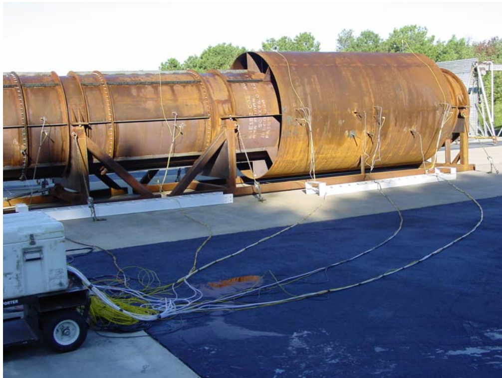
Figure 3.24 Installed Temperature, Pressure, and Vibration Measurement Cables.
