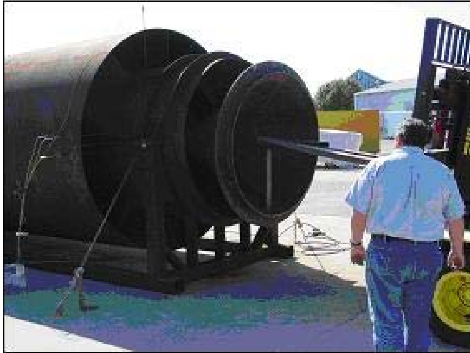
Figure 3.19 NADc “Cone” End-Piece Being Inserted into NAD for Attachment.
