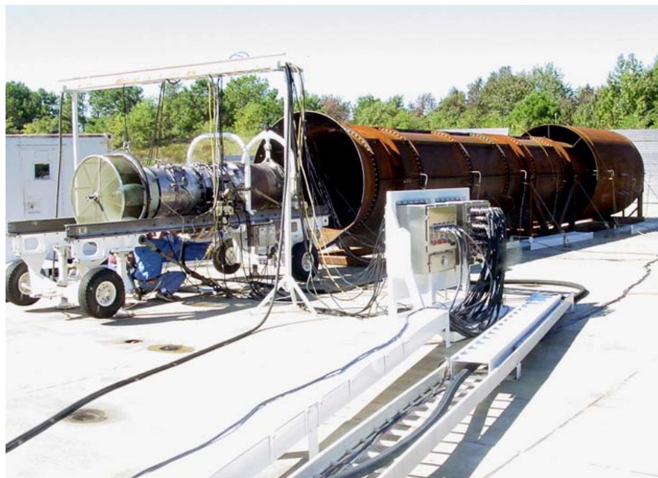
Figure 3.14 NAD Installed for Testing with J-52 Engine – No Flow Deflector.
