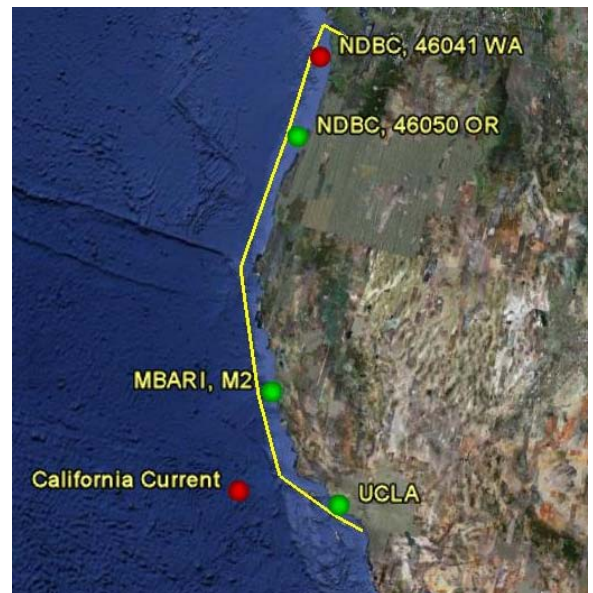
Fig. 8 In Year 3 of the project, a second Wave Glider will execute an extended (>2000 km) autonomous mission (yellow line) to measure coastal carbon chemistry parameters along the west coast of the US.
