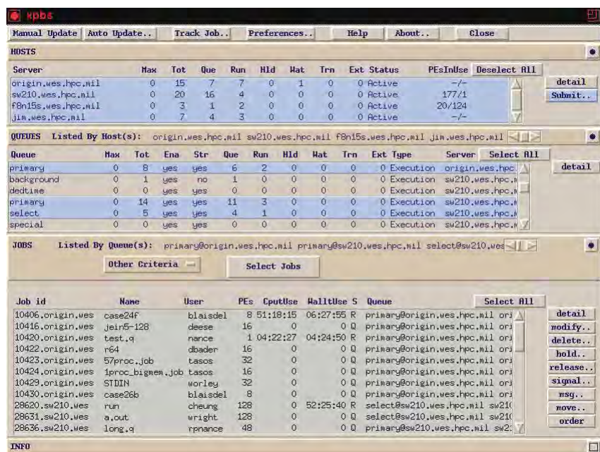
FIGURE 1. The PBS graphical user interface, xpbs, offers a single interface to different supercomputers which allows the user to select which queues and jobs to display, while providing point-and-click batch job submission.
