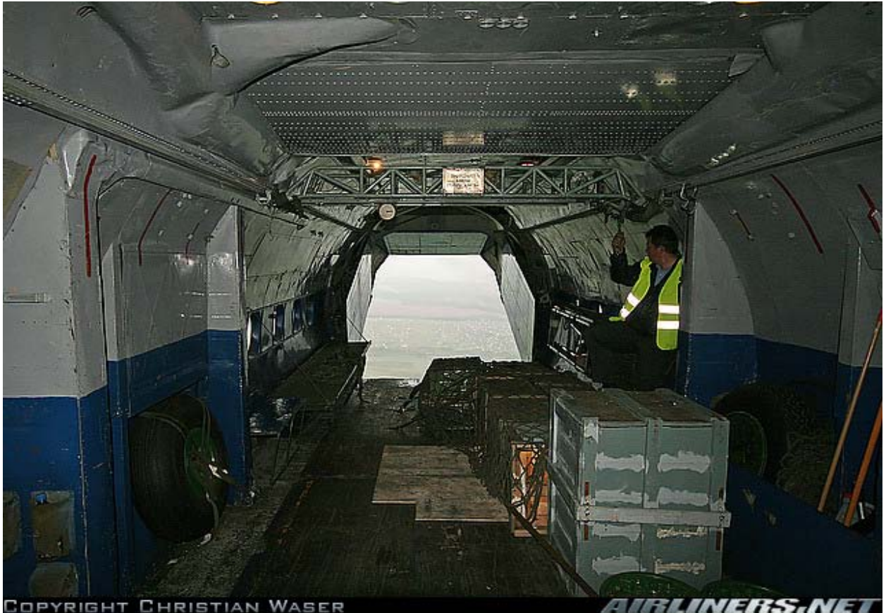
Interior of An-12 with rear door open in flight for demo. Note overhead crane, wood floor, and lack of rollers. Copyrighted image used with permission.
