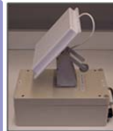
Tracking antenna and Wave Relay mesh link
